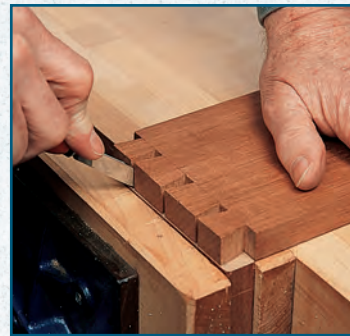
Mark the pins from the tails with a marking knife.
