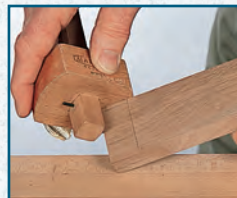
Set the mortise gauge with the chisel you'll to chop the mortise (top right), then mark the tenon edges and end with your mortise gauge (above). Turn to the marking gauge (bottom right) to mark the tenon sides and end.
