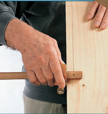
A marking gauge cuts with the grain. Note the basic gauge grip — thumb behind the fence, index finger over the fence, three fingers grip the stock.
