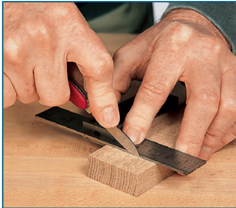
A rounded knife produces a smooth cut because pressure is distributed over a curved edge rather than concentrated at the point.
