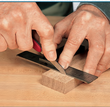
Knife the tenon's first shoulder. Use the face side and face edge to continue squaring round. For the second cut, rotate workpiece 90°. Mark the second set of shoulders from the first set.
