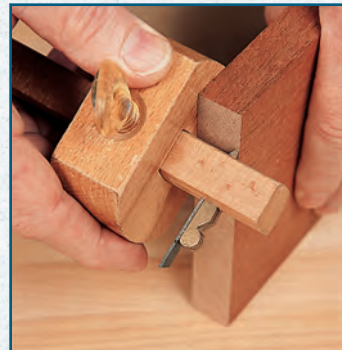
Set the cutting gauge 1/32" less than the thickness of the pin piece.
