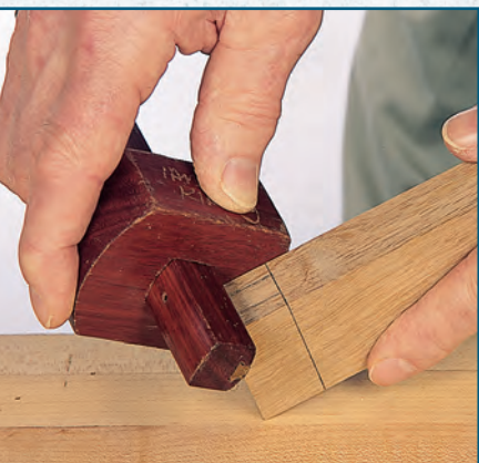
Set the mortise gauge with the chisel you'll to chop the mortise (top right), then mark the tenon edges and end with your mortise gauge (above). Turn to the marking gauge (bottom right) to mark the tenon sides and end.
