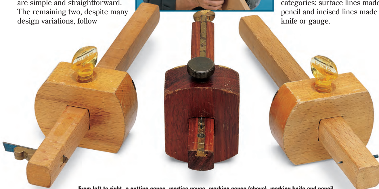
From left to right, a cutting gauge, mortise gauge, marking gauge (above), marking knife and pencil (below) are the tools author and master craftsman Ian Kirby uses to mark out precise joinery.
