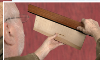
Checking straightness on the face edge of a board with a wooden straightedge.
