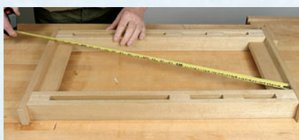
Checking squareness of an assembly with a tape measure.
