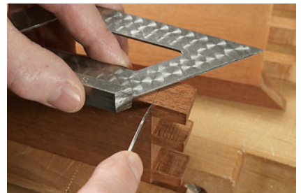
Position your marking knife in the line on the face of the workpiece, then slide the miter square to the knife.
