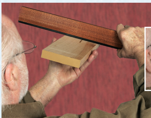
Checking straightness of the face side of a board with a wooden straightedge.
