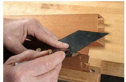
You have to position the knife where you think the miter will fall, then slide the square to it. "Sometimes the magic works; sometimes it doesn't." — Little Big Man.
