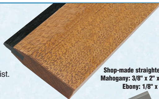
Any inaccuracy in the squared edge is augmented when the blade is placed across the side instead of the edge.
