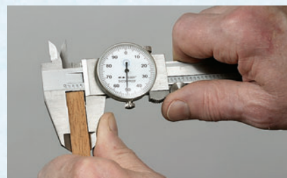
Use your thumb to firmly press the fixed jaw into full contact with the workpiece.
