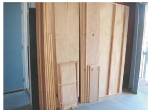
I also attached two long horizontal 'ribs' to the Back Panel 'C' (which can be seen above on the right) to support the center and lower shelves ('E' and 'F'), since the back pair of dowels do not go all the way down. (See Step 5).
