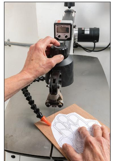
**5. Problem: Excess burning when cutting thick or dense wood.** *Possible causes:* wrong size or type of blade for thickness or type of wood.
