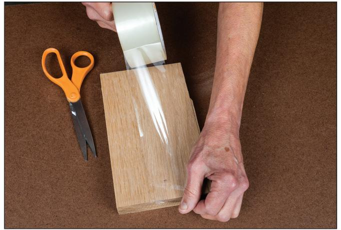
*Applying tape to the workpiece provides lubrication for the blade and makes it easier to cut wood that is hard, dense or burns easily, like cherry. Blue painter's or clear packing tapes are popular choices.*
