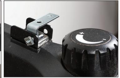
*Scroll saw angle gauges, located below the saw table, are awkward to read and inadequate when accuracy is important. A digital readout is more precise. It can be used with all types of scroll saws, placed either on a tilting table or saw blade, or attached to a tilting arm.*
