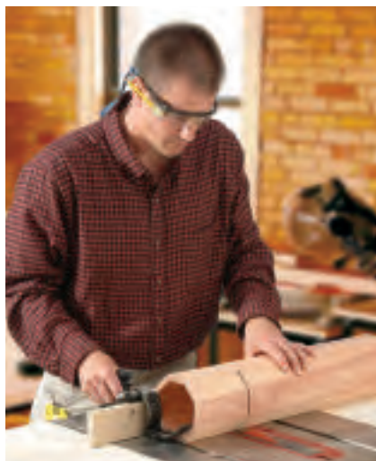
Absolute accuracy is never in doubt if you make your canisters from one glued-up octagon. A flip-stop miter attachment makes it easy to crosscut the canisters accurately. (If you don't have a flip stop, attach a scrap stop to your miter gauge instead.)
