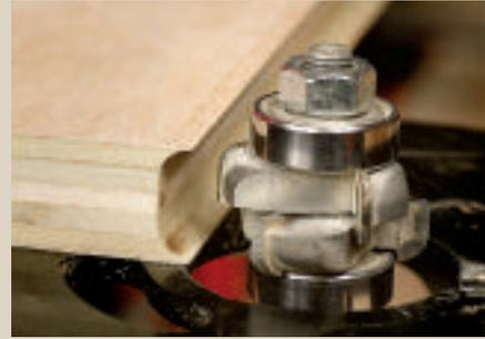
*The Burgess Edge plywood bit has two stacked, adjustable cutters that scoop out the panel edge, leaving a knife-edge of hardwood veneer.*
