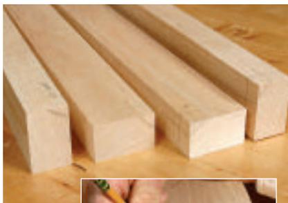
Identify and orient the front and back legs. Mark locations for the top rail mortises (except where the top front rails join the legs). The author chose pocket joints for that task.
