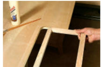
Machine the desktop cutout with the Burgess Edge plywood bit and the newly shaped infill frame with the Burgess insert bit. Apply glue and slide the frame into the cutout.
