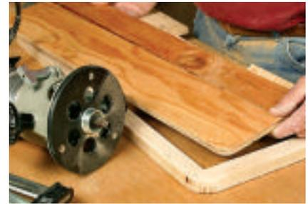
The secondary template the author is holding was used to shape the edges of the infill frame that was assembled with half-lap joints. The template was screwed in place with about 1/2" of the frame exposed on three sides. Then it was a simple matter of routing around the template to trim the frame to exact size.
