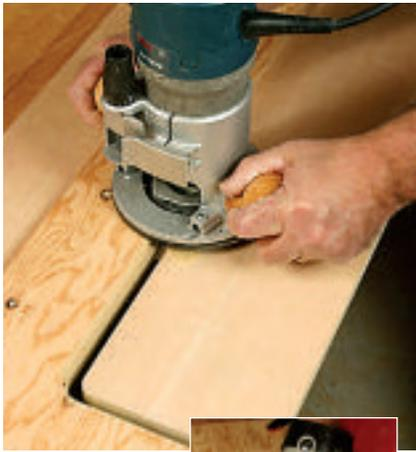
Use your master templates (the author used a good size Forstner bit to form the corners) to form the cutouts in the desktop (far left). The templates will guide a router fitted with a 3/4" template guide and 1/2" compression bit. Then, use the same templates to create secondary templates (left). For this step, clamp the master to your plywood and guide a router fitted with a 3/8" template guide and 1/4" straight bit along the edge.
