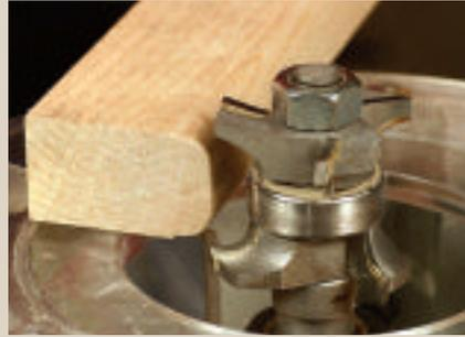
*With its center bearing and a little fine adjustment, this bit forms perfectly sized hardwood edging with plenty of glue surface.*
