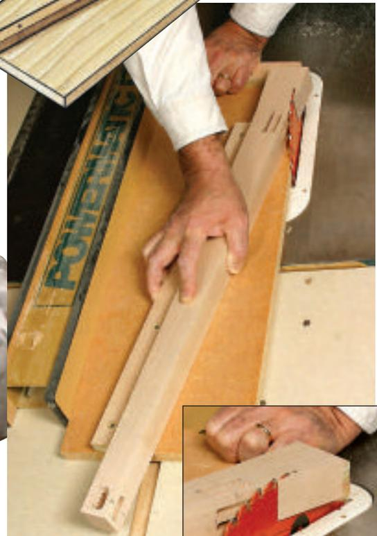
*Saw the inside foot taper to avoid major tearout problems. Attach a couple of fences to a scrap panel to make the jig quickly. Recycle the screws and panel after the legs are cut.*
