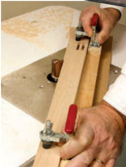
Attach fences to the leg template, and mount a couple of toggle clamps on them to secure the leg blank. Band-saw off the majority of the waste, then template-route the leg flush using a bearing-guided bit.
