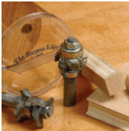
*The patented Burgess Edge is created with these two, two-part router bits. Using this system to put hardwood edges onto veneered panels has several advantages.*
