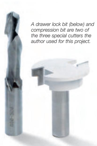
*A drawer lock bit (below) and compression bit are two of the three special cutters the author used for this project.*
