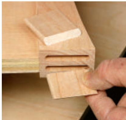
Before you begin the final pedestal glue-up, glue the loose tenons into the rail mortises. Be sure you orient the bevels properly.
