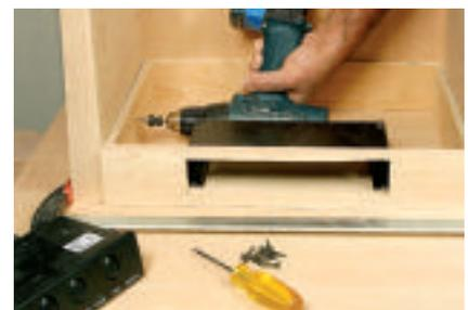
The Power Director (shown in photo) is mounted in a frame at the bottom of one of the gallery towers. The frame is screwed to the side of the tower and a port is cut in the desktop for cables. A removable shelf hides wire clutter.
