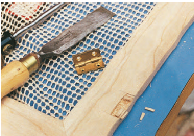
Marking out and chopping the hinge mortises was a hand-powered operation. The author's wheeled scribe and a sharp chisel made short work of the three-step process.
