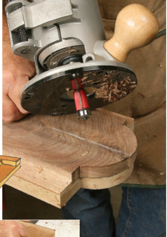
The tombstone panels (and the rail that receives them) require some template routing. When raising the curved ends of the panel, use a safety block to apply downward pressure.
