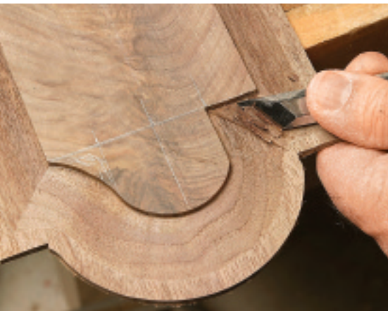
After squaring up the inside corners of the field with your bench chisels, switch to skew chisels—first right and then left—to finish the fillet.
