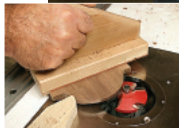
The tombstone panels (and the rail that receives them) require some template routing. When raising the curved ends of the panel, use a safety block to apply downward pressure.
