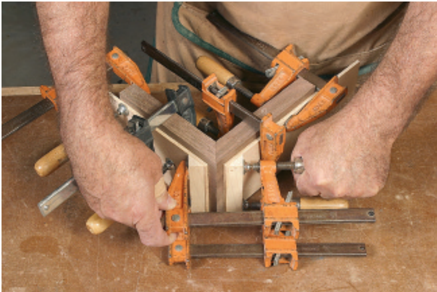
The author made some handy clamping cauls to help hold the mitered foot joint firmly. The triangular blocks are glued to 1/4" plywood. The plywood is clamped to the foot blank and pressure is applied to the triangular blocks. Easy and effective.
