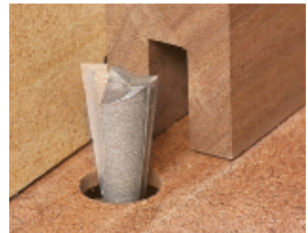
After plowing a 5/16" groove centered on the edge of the breadboard ends (to remove most of the waste), the author formed a 3/4"-deep dovetail groove.
