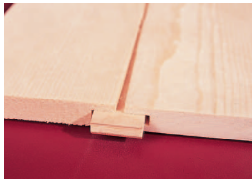
Figure 7: The 1/4"-thick splines in the back are cut from scrap plywood. Solid-wood splines would just crack along their grain.
