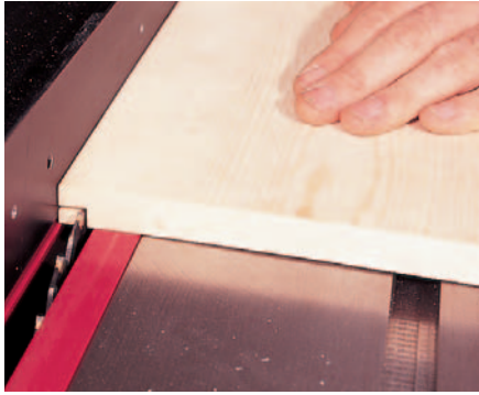
Figure 1: In the traditional mode, we glued up solid-wood panels for the sides instead of substituting plywood. Rabbits for the back were then cut on a table saw, as shown here.
