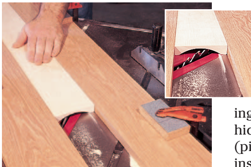
Figure 5: To create the cove molding, use your miter gauge to orient and clamp fences at 45° to the blade, then raise the blade 1/16" per pass as you cut the curved profile.
