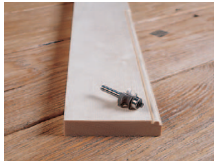
Figure 4: To create the traditional decorative detail on the edges of the stiles, use a bearing-guided beading bit in your router.
