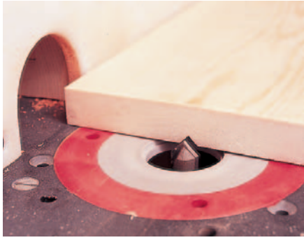
Figure 3: To display your best pewter, cut plate grooves in the shelves with a V-groove bit in the router table.
