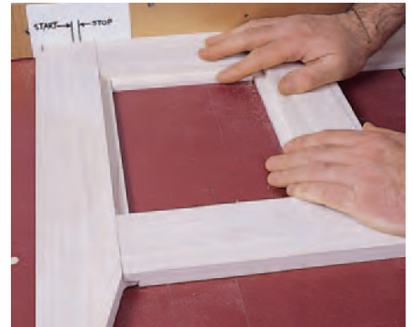
Figure 2: Align marks on your router table fence and the stiles to locate the two stopped dados that will hold the bottom panel.
