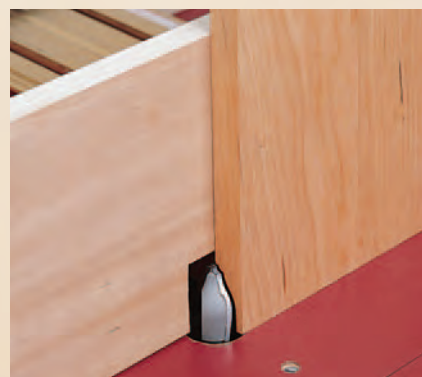
The keys to using vertical panel raising bits are to support them with an auxiliary fence on your router table and to take multiple light passes.
