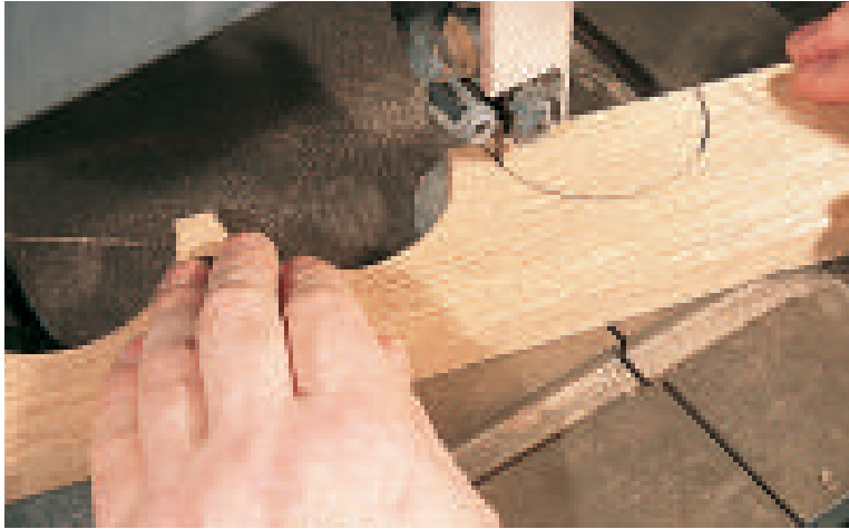
Figure 5: Slice the large semicircles in the back racks on a bandsaw, then remove the kerf marks with a drum sander.
