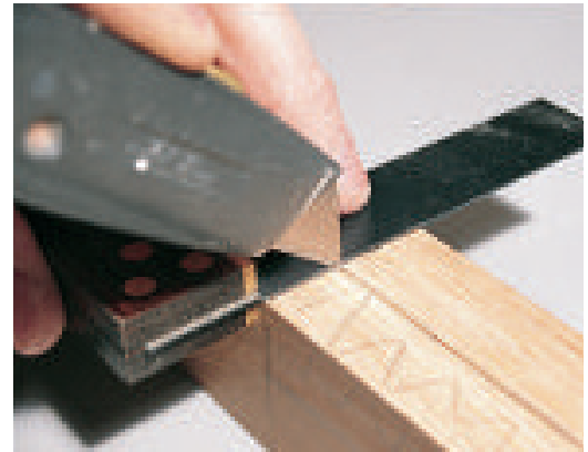
Figure 2: To stop chipping and tearout, use a sharp utility knife to score across the grain at each end of the stopped rabbets.
