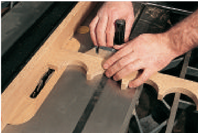
Figure 6: Use your table saw to cut shallow rabbets into each end of the front and back aprons and the lower racks for attaching these parts to the legs.
