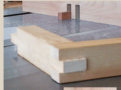
Using a registration pin mounted in a backer board, the author made a "one-time" finger joint jig for his table saw.
