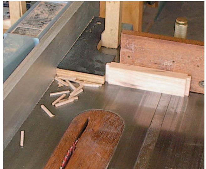
Using a stand-off block to register the cut and a miter gauge for safety, machine tenons onto the ends of the muntins.
