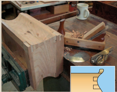
The lower bout of the S curve is started by slicing an angled cut at the bottom edge of the box, as shown in the inset.
