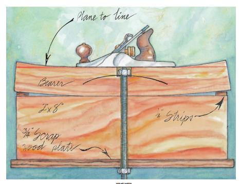
Make a stand out of the 2" x 8"s for bending the first bearer. Stand them on top of the plate, then slip a threaded rod through the bearer, between the 2" x 8"s and through the plate hole. Place the 1/4"-thick strips beneath the bearer, add the washers and tighten the nuts until the bearer touches the 2" x 8"s.
