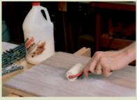
Use a small roller to spread glue evenly on the substrate. To avoid excessive curling, don't put glue directly on the veneer.
