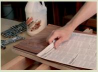
Place the veneer on the substrate, then lay newspaper down to keep excess glue from bonding the cauls to the veneer.
