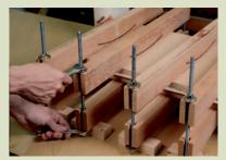
Tighten the nuts with a box wrench until you see a consistent bead of glue squeeze-out along the edges of the panel.
