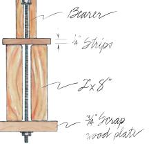
then return the bearer to the fixture, tighten the nut and hand-plane the edge right to the line. Since the camber is so subtle, draw a large curved line on the side of the bearer to indicate the correct edge.
