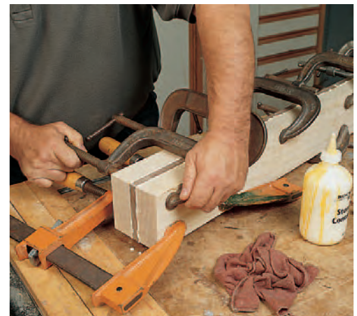
Glue the leg laminations together, holding the parts with plenty of clamps until the glue sets. Check the joint initially to remedy any glue creeping.
