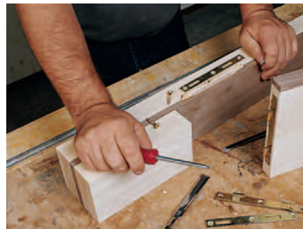
Installing knock-down bed rail hardware in mortises keeps it invisible when assembled.
