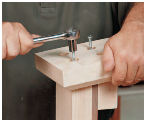
Heavy-duty lag bolts ensure that the arched pediments will not come loose from the bed's legs. Make sure you sink the heads below the level of the arch.
