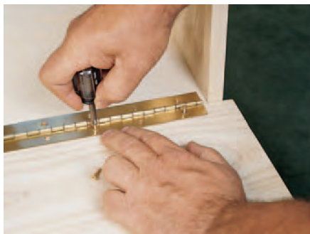
Sewing machine hinges were tested, but they weren't up to the job. Piano hinges offer the strength and support these doors need.
