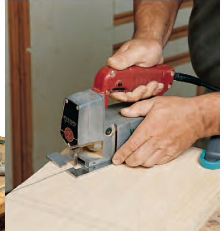
Get close to the layout lines for the side with a hand-held jig-saw. Then finish the cut with a router and a straightedge jig, (left), to smooth the saw marks.
