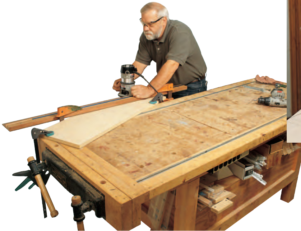
Use a straightedge jig and a router with a straight bit to trim the angled front edges smooth and straight.
