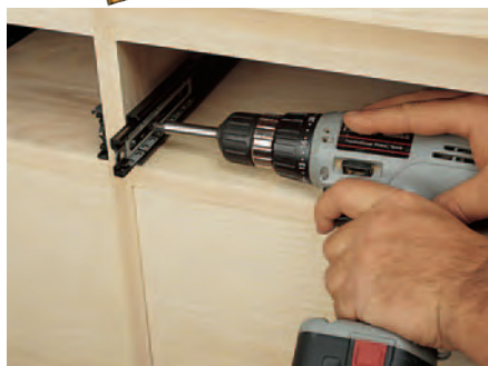
Putting It All Together. Heavy-duty drawer slides are an important feature, as the drawers (when open) do double duty as door supports.
