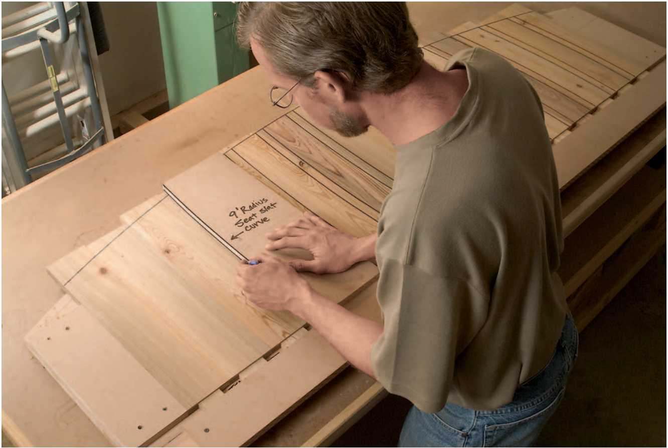
Drawing parallel curves on the back slats is easy if you group the slats together in a jig. Make a template with a curve based on a 9-foot radius, and trace the curves onto the slats using the template. Shape the slat jig so the top edge matches the crest rail mortise curve. This way, you can scribe the slat top curves as well.
