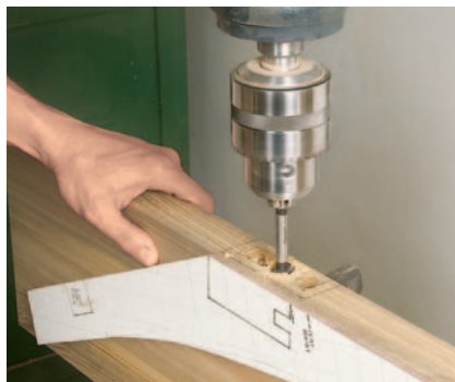
The author fixed a leg template to each leg blank and left it there for the entire machining process. Drill the mortise for the seat rail before you cut the back leg out of its blank.
