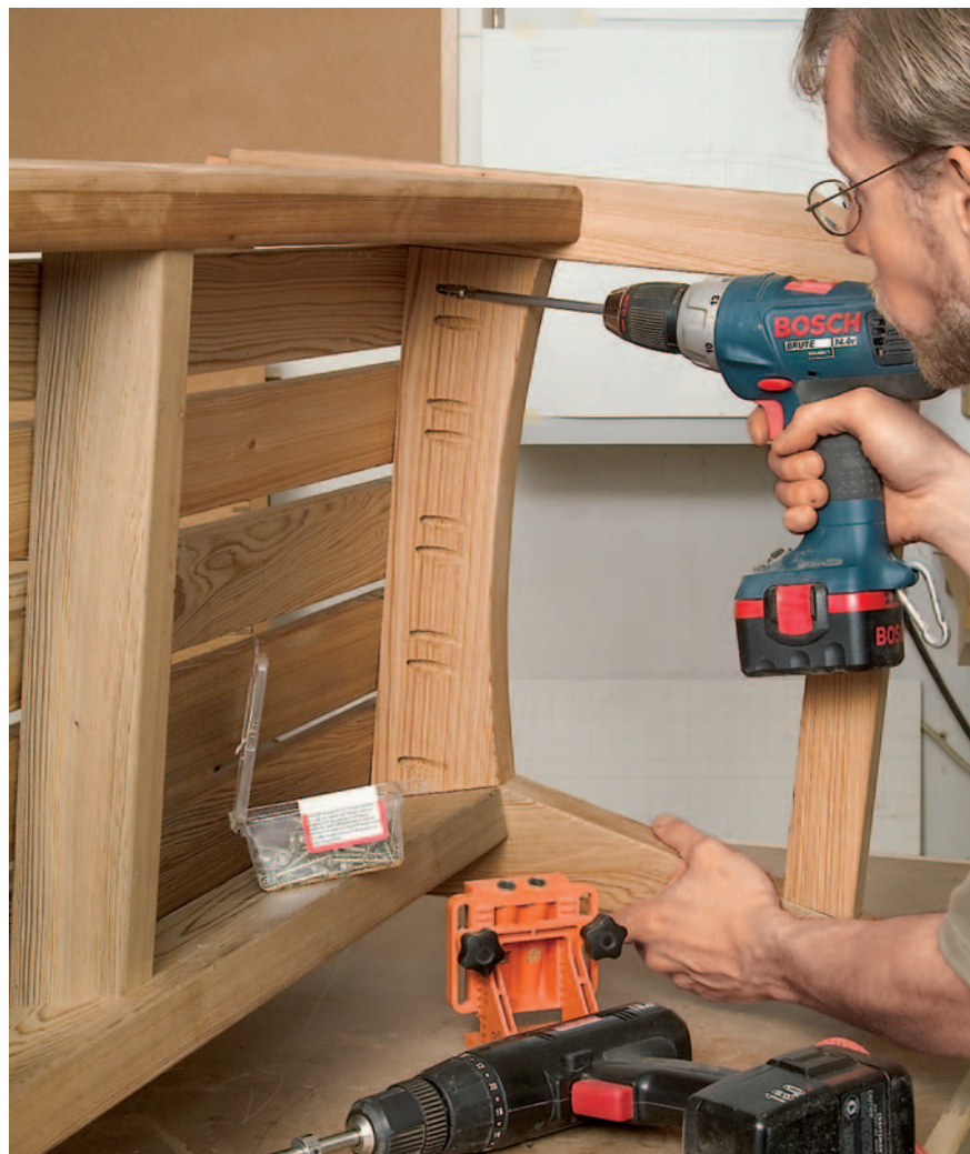
To hide the seat slat fasteners, drive them in from underneath. The author used a pocket-hole jig and weather-resistant pocket screws. Tack the slats in place first with glue.
