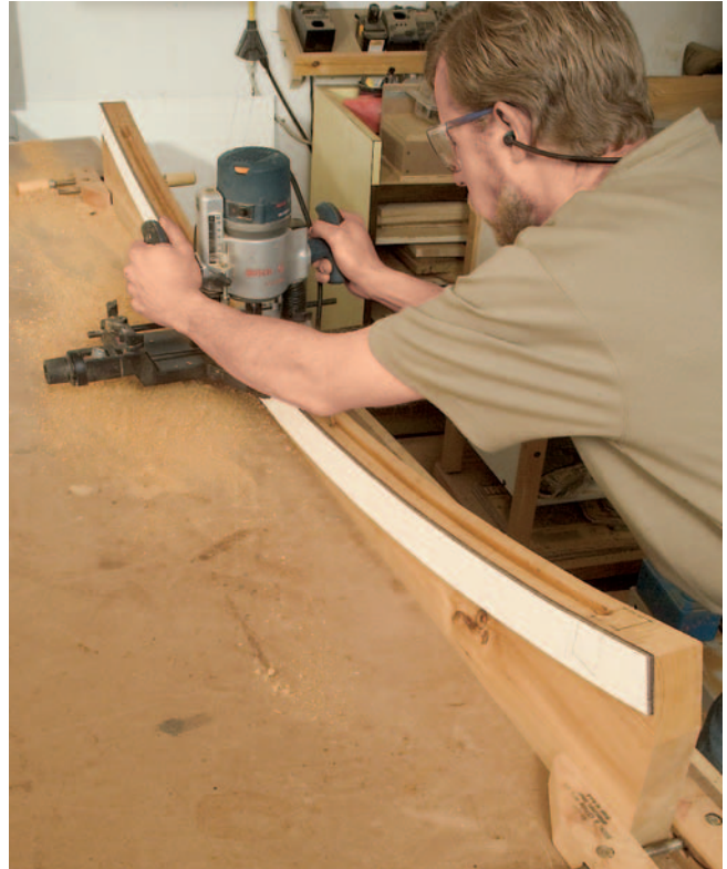
Rout the shallow step of the crest rail's continuous slat mortise first. Plow it from one back leg mortise to the other. Then mill the 3/4"-deep stopped portion of the slat mortise with the same bit and edge guide setup.
