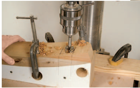
Cut out a portion of your full-sized bench end view pattern to make an alignment jig for drilling the armrest mortises. The goal here is to cut these mortises so the legs meet the armrests squarely, despite the curve.
