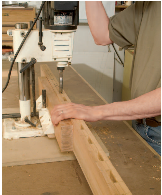
The back slats fit into individual mortises in the back rail. A hollow chisel mortiser is the perfect tool for this repetitive chopping task. Or, you could cut them with a plunge router fitted with an edge guide.
