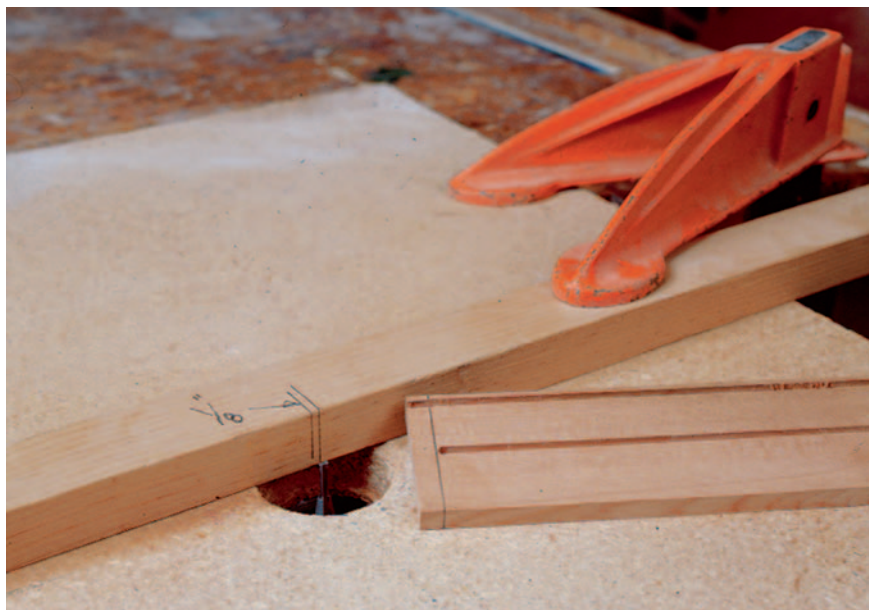
Figure 1: Outline the bit's cutting area on the fence, then use the lines as starting and stopping points when routing the stopped grooves.
