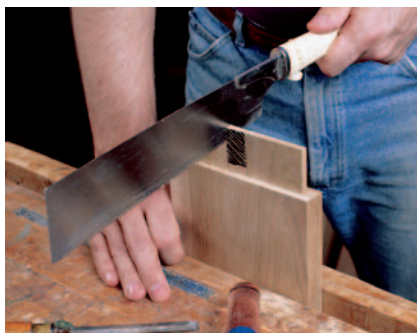
Figure 5: Once you've formed the tenons with your table saw, dado blade and miter gauge, cut the gap in each lower rail tenon with a hand saw.
