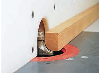
Figure 4: The outside edge of the large door molding is shaped on a router table with a 3/8"-radius roundover bit.
