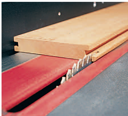
Figure 5: The safest way to make the small quarter round molding for the door edges is to form it first with a router on the edge of a wide board, then rip it to width as shown here.
