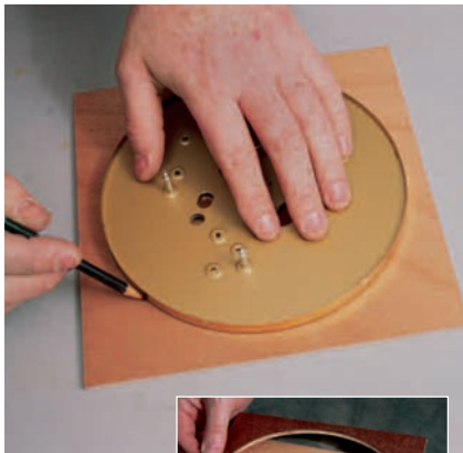
Figure 8: A 1/4" plywood template will help you place the clock face accurately.
