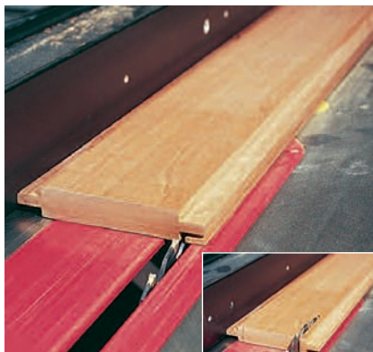
Figure 6: Machine the muntins from larger pieces of lumber in a two-step process.
