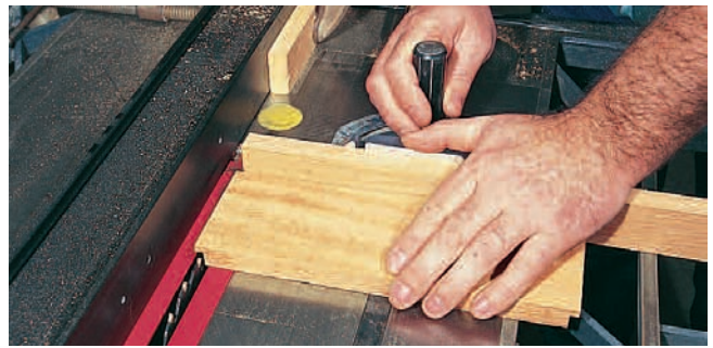
Figure 2: Tongues on the top and bottom fit into dado slots in the sides. Create them by milling rabbets on the opposing edges.
