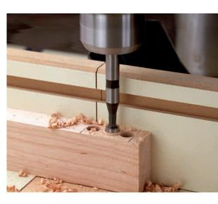
Pare the walls of the mortise smooth and flat with a couple of sharp chisels. It's best to make the mortises first and then form tenons to fit the openings.
