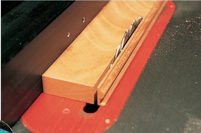
Figure 2: The safest way to make your small moldings is to rout the profile on a wider board, then rip off the edge on your table saw.
