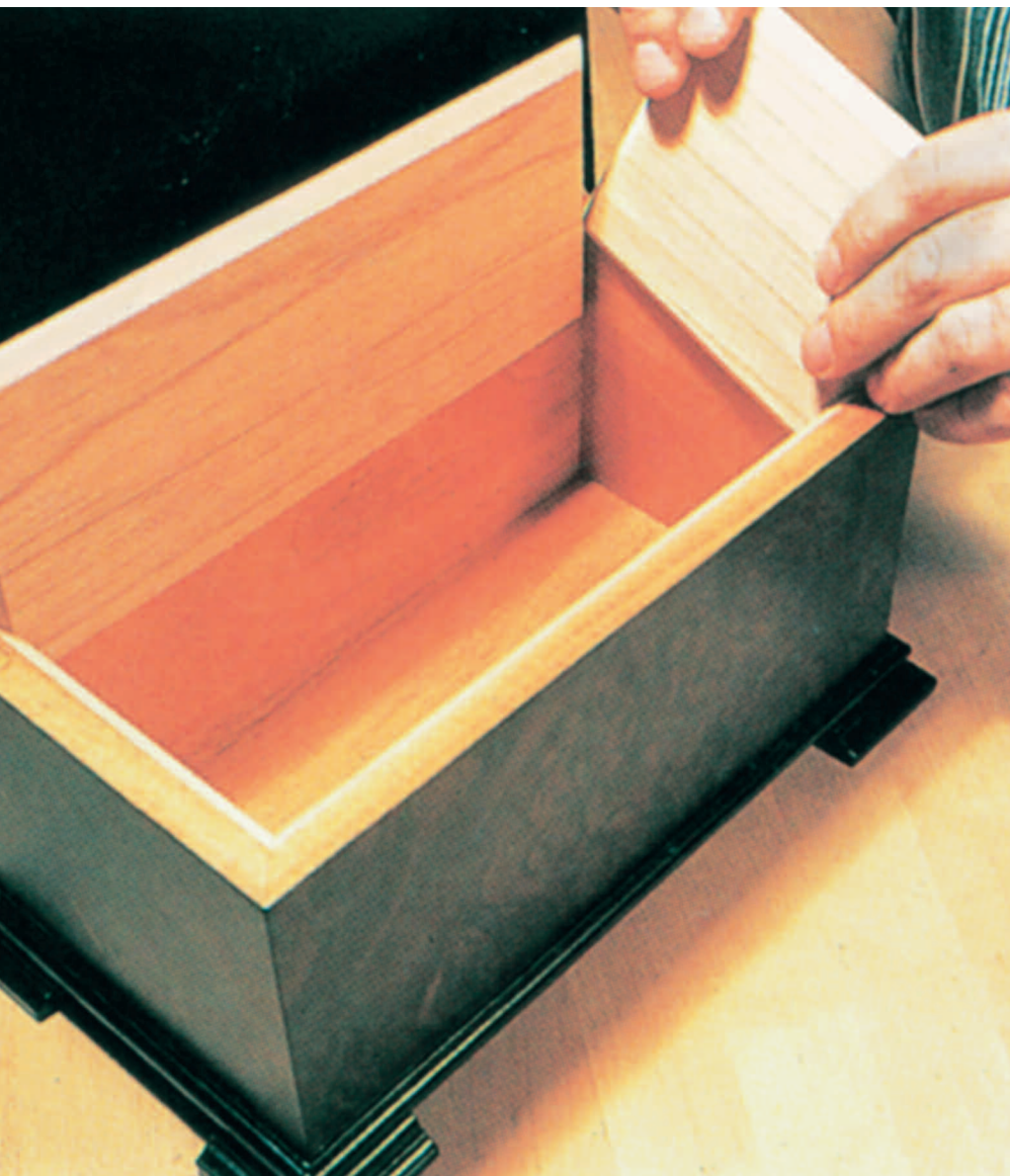
Figure 4: Drop the Spanish cedar bottom and sidewall liners in place, but don't glue them in so you can replace them in a decade or two.
