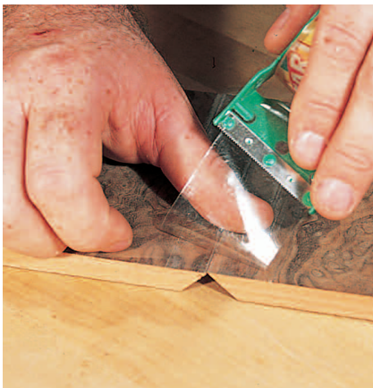
Figure 1: Clear strapping tape is the perfect clamping solution when it comes to applying equal pressure to mitered box sides.
