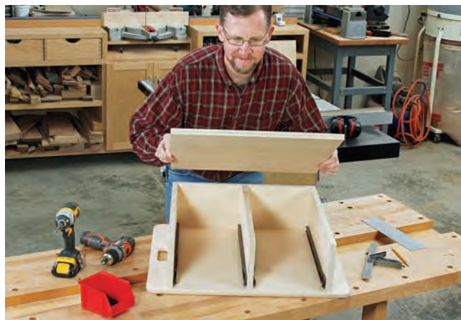
Install the drawer slide hardware before assembling the sides, divider and back panel on the base. The roller tracks would be much harder to install after you've undertaken the assembly.
