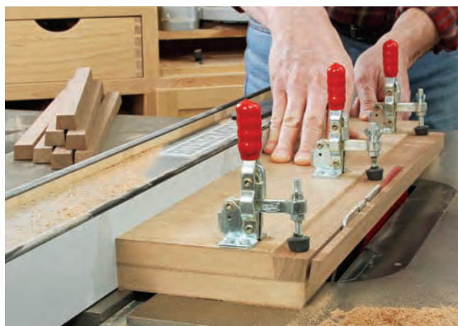
The author made a simple ripping jig to secure each dovetail extension strip for cutting its second beveled edge. Toggle clamps make for quick changeovers and keep fingers a safe distance from the blade.
