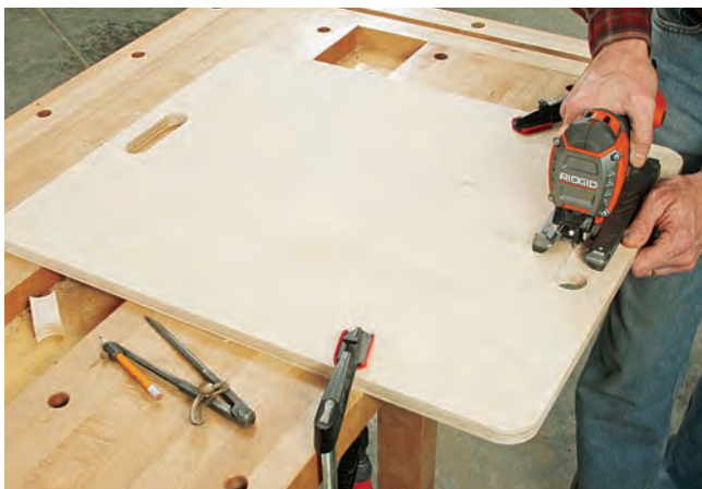
The author used just two lifting handles, but four (two per side) would be useful if you have a heavy mortiser needing two people to carry it. Use a Forstner bit, then a jigsaw to create the cutouts.
