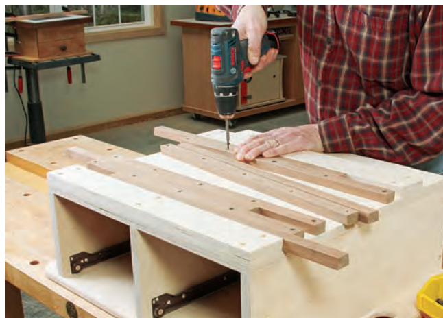
Arrange two groups of four dovetailed extensions against the machine bases with their bevels alternating and engaged. Fasten four strips to the carcass top to create "tracks" for the other four strips that slide.
