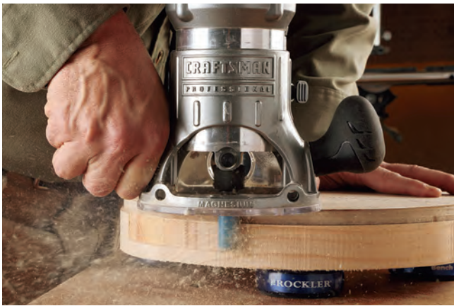
The author used a 1/2"-thick MDF template and a handheld router outfitted with a pattern-routing bit to make identical seat components. Later, the edges of the appropriate pieces were rounded over.
