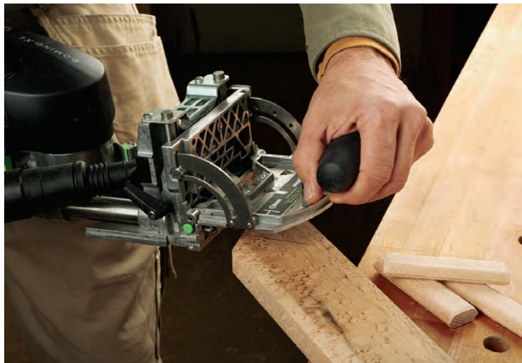
Cutting the mortise for the thick and strong Domino loose tenons is a matter of lining up the machine to a line. The adjustable horizontal fence on the machine locates the mortise in the center of the stock.
