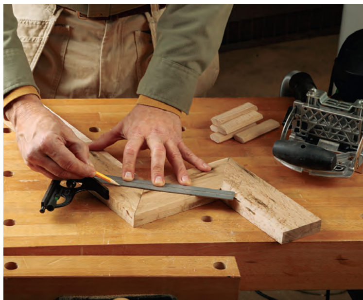
The mitered legs are made and glued up in sections. Here, the lower leg and crosspiece have been glued together. The author is marking the loose tenon location for the upper leg and lower section subassembly joint.
