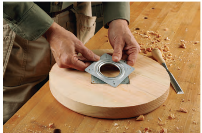
The author's coworkers thought that the seat should swivel and spin, so he added a lazy Susan to the last layer of the seat sandwich. The recess needs to be slightly less deep than the bearing's thickness.
