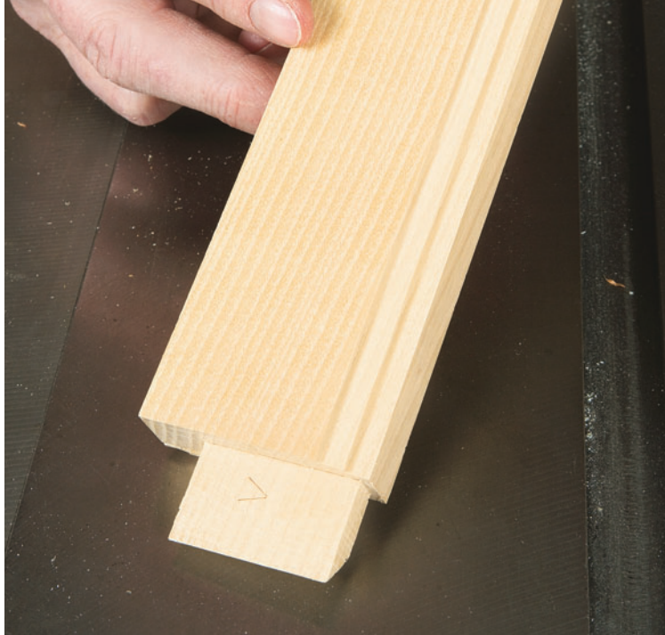
To form the rabbets on the rails, the author used a cleaned Freud combination ATB blade with every fifth tooth a flat top. These shapes are purposefully placed to create depth through the interplay of light and shadow.
