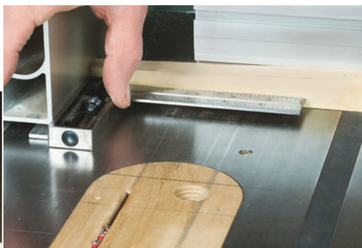
With the saw blade set at 3/32" above the table, incise rabbets to form the foot. The author describes the cutting sequence in the text "Shape the Foot."
