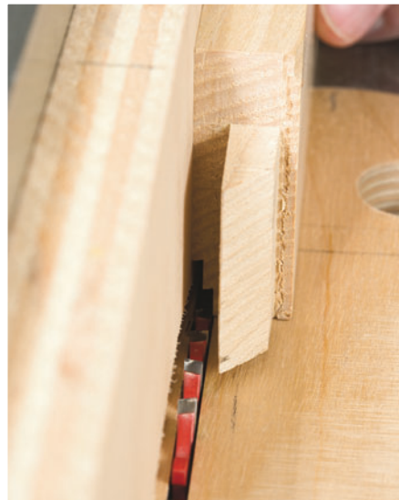
To form the rabbets on the rails, the author used a cleaned Freud combination ATB blade with every fifth tooth a flat top. These shapes are purposefully placed to create depth through the interplay of light and shadow.
