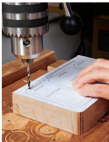
After cutting the box's outer profile to shape, drill a starter hole in the insert area of the pattern to thread your blade through. Then cut out the large inside waste piece with a #9 blade. Consider saving the waste piece for a future project.
