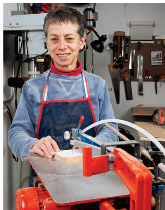
After cutting the box's outer profile to shape, drill a starter hole in the insert area of the pattern to thread your blade through. Then cut out the large inside waste piece with a #9 blade. Consider saving the waste piece for a future project.
