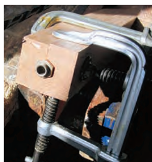
Glue up the stem flat on the workbench with a 6" length of 3/8" threaded tubing in place. It took multiple clamps to get good pressure along the length of the stem to create a tight seam.
