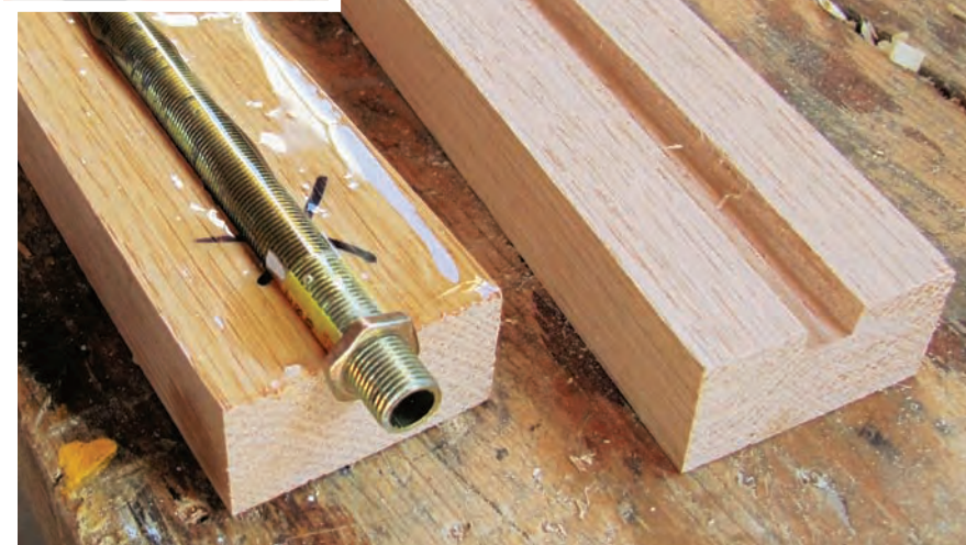
The author formed the opening for the threaded tube and lamp wire by making multiple cuts on his table saw (top photo). A dado head would work well, as would a router — he had neither. Lay the threaded tubing in place before gluing up the stem. Leave enough of the tube projecting so there is room for the shade support (or “harp”), a second retaining nut and the bulb holder. The author used epoxy as his adhesive, but any good quality wood glue would work as well.
