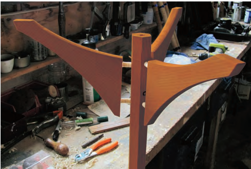
It is important to test fit all the parts. The author located the dowel holes on the stem by pre-drilling holes in the feet and then using dowel points to transfer their positions.
