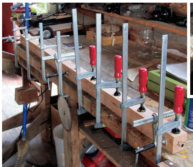
The author formed the opening for the threaded tube and lamp wire by making multiple cuts on his table saw (top photo). A dado head would work well, as would a router — he had neither. Lay the threaded tubing in place before gluing up the stem. Leave enough of the tube projecting so there is room for the shade support (or “harp”), a second retaining nut and the bulb holder. The author used epoxy as his adhesive, but any good quality wood glue would work as well.
