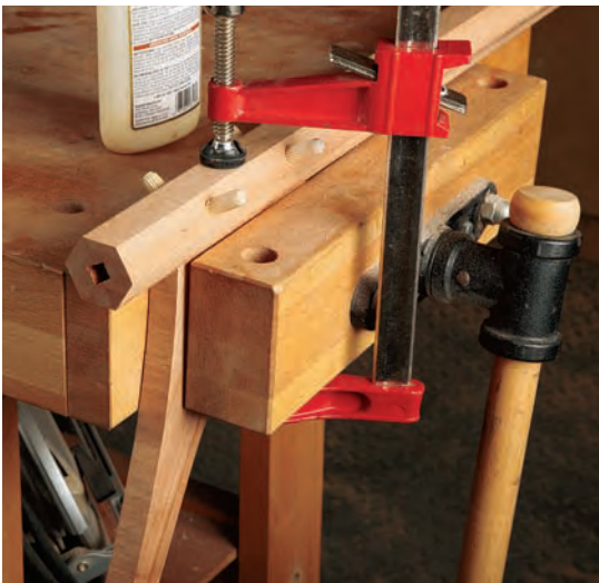
To clamp the feet securely, place one in the vise, apply the glue to the dowels and the stem, then clamp down to the vise. This makes an otherwise awkward process much easier.
