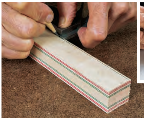
Mark layout lines (left) for cutting strips of 1/16"-thick ribbon (top). Before sawing, sand the blank to smooth one of each ribbon's faces.
