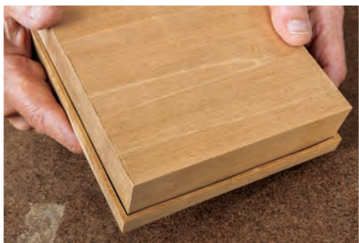
Smooth and square up the box lid with some careful work at the disc sander (right). When fitted on the box (above), the lid should slip into place with minimal side-to-side play.
