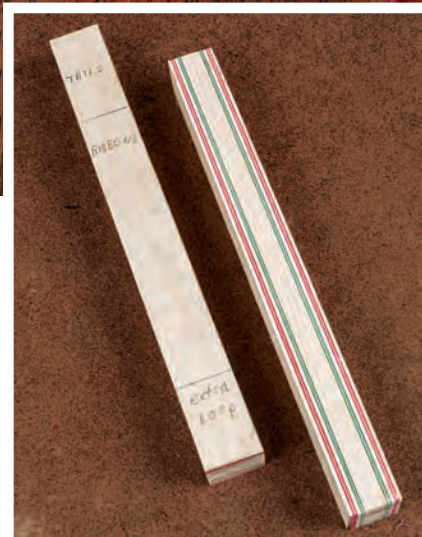
Multiple laminations of clear maple and both dyed and plain veneer form blanks for the patterned ribbons, bow loops and tails.
