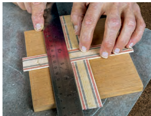
Glue and clamp one ribbon across the top of the lid, and clean up any squeeze-out (top). Line up and glue on two more ribbons to form a crisscross pattern (bottom).
