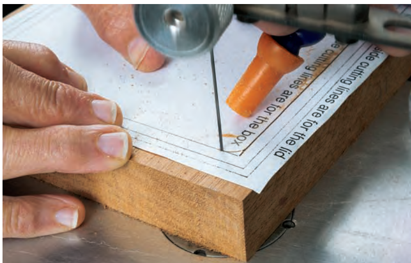
Mount the paper pattern (page 4) to a 1"-thick square of mahogany that will become the walls of the box. Cut along the inside line to remove the large center waste piece.
