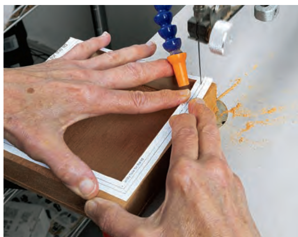
Cut along the pattern's middle line to reduce the box walls to 1/8" thickness and to trim the box to final size. Already installed, the bottom will match perfectly.
