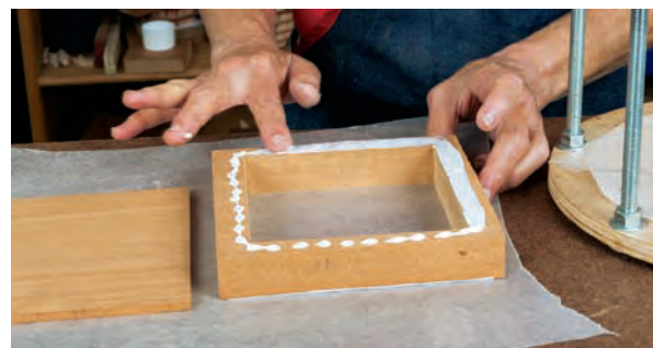
Spread glue around the bottom edges of the box wall workpiece, and clamp on the 1/4"-thick bottom panel.
