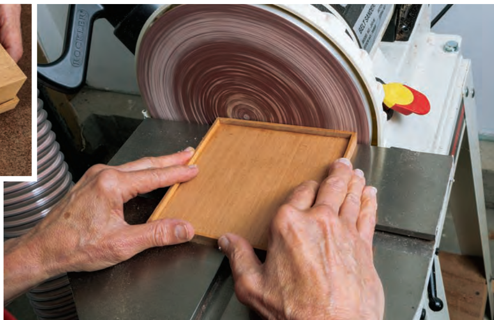
Smooth and square up the box lid with some careful work at the disc sander (right). When fitted on the box (above), the lid should slip into place with minimal side-to-side play.
