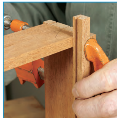
The proper position of the drawer slip is tight to the side, engaged in the drawer front's groove and snug to the bottom edge of the back.
