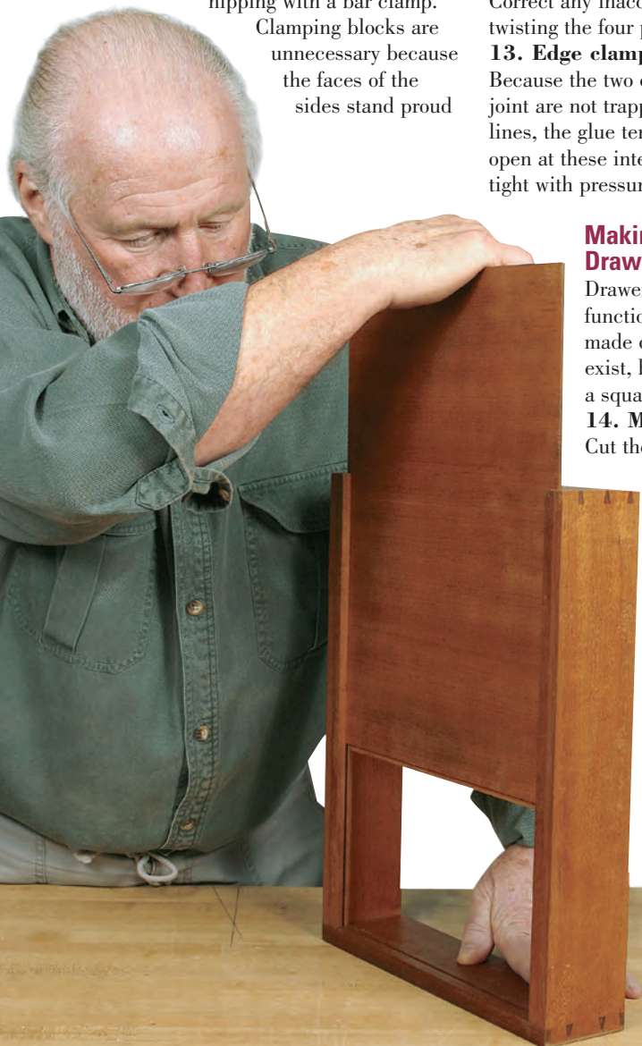
To create the second tongue on the drawer bottom, establish the shoulder with a knife line. Cut all tongues with a shoulder plane.
