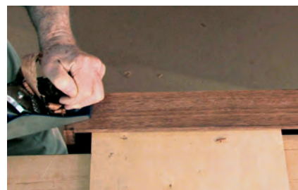
Hang the drawer side on a board that is clamped securely to the bench top. The front of the drawer is held tightly in the vise.
