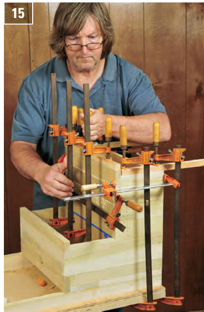
Glue-up of the step stool takes place in four stages, as described in the story below. The author notes that you must take care to keep your pieces flush; small brads snipped off close to each mating surface (as shown in photo 10) help to prevent pieces from sliding.
