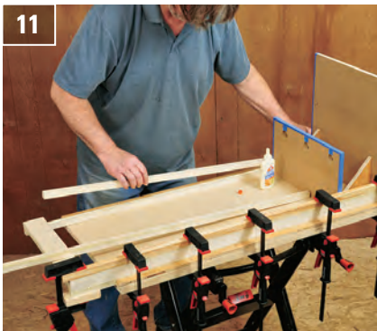
Glue-up of the step stool takes place in four stages, as described in the story below. The author notes that you must take care to keep your pieces flush; small brads snipped off close to each mating surface (as shown in photo 10) help to prevent pieces from sliding.
