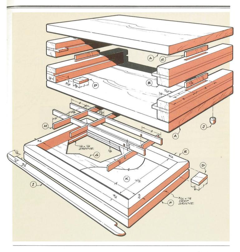
nently in place; the stops prevent them from pulling all the way out. But first you'll want to make sure that the drawers slide easily. This may take a little hand sanding to thin and shorten the stops, if they are binding in the grooves. Add a little paraffin wax to ease the drawer action.
