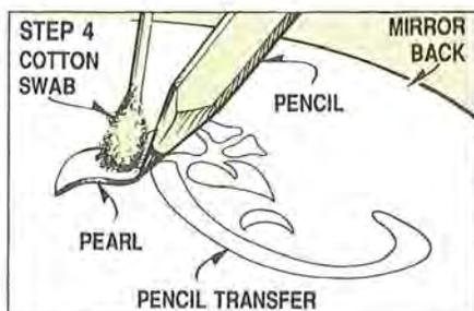
best to have the ground—in this case the back of the mirror—clamped securely to your bench top so it won't be moving about as you trace the pearl.
