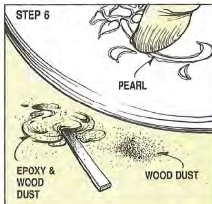
Press in the sections of pearl as shown. Don't dally here since the epoxy will start to set up. For larger patterns you may want to work on only a few parts at one time, or you can switch to a standard epoxy with 24-hour dry time. Press in the sections of pearl until they bottom out. The excess epoxy and wood dust mixture will be oozing out all around the edges, but don't worry about that now. You'll sand the excess off after it dries.
