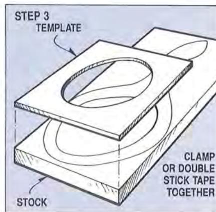
to the stock, but keep the clamps close to the corners so as to not interfere with the router base. Doublestick tape or countersunk screws are an option if the clamps interfere with the router.
