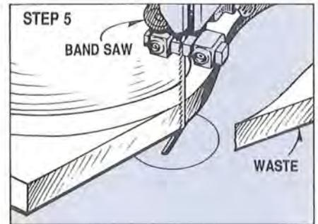
**Step 5:** Cut the outside profile. Use the band saw, handheld jigsaw or a coping saw. Use files to smooth any irregularities and remove the saw marks. It's important that the edge be smooth for the next step.
