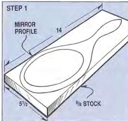
be sure to also cut out the center, since you need to mark the mirror glass position on the stock. When making multiples, a cardboard or hardboard template simplifies the task of transferring the profile to your stock. An easy way to get the full pattern of the mirror body is to just fold the photocopy along the center line, cut and unfold. Note that the contoured handle is for a right-hand grip. Reverse the pattern for a left-hand grip.
