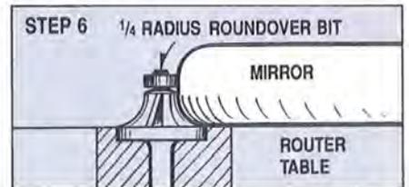
**Step 6:** Radius the edges. We used the router table with a  $\frac{1}{4}$  in. radius ball-bearing guided roundover bit. Round one edge, then flip the mirror over to round the other edge. Final sand with 320-grit sandpaper.
