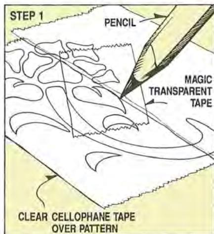
But with our technique you can reuse the original pattern as many times as you wish, without damage. Start by taping over the original full-size pattern with clear cellophane tape as shown. You can
