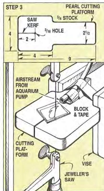
enough tension to keep the blade from buckling, but not so much as to place the blade under stress where it's liable to break easily.
