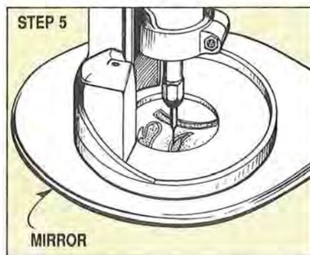
the 1/16 in. solid carbide inlay bit. The bit depth of cut is set just a hair under the pearl thickness, allowing the pearl to stand a little proud of the ground's surface. Note that on our bit we had to grind the end of the shank back slightly to get the proper depth setting in the collet.
