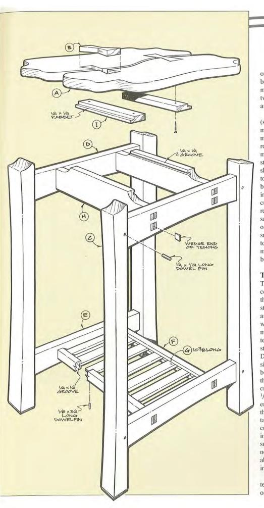
of the top together with the strips between; the three 1/8 in. strips will maintain the 3/8 in. spacing between the two halves while the butterfly mortises are cut.
