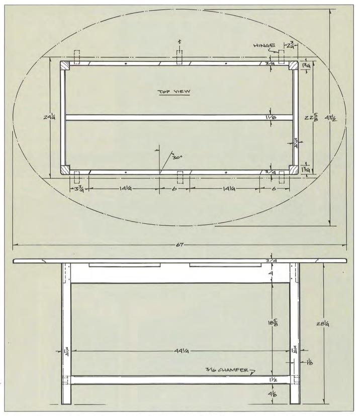
If the action is smooth, now lay out the oval shape (see Making The Oval) and cut the edge. The easiest way to get a good, even edge all around is to use the oval layout instructions to make a hardboard template that's just a little larger than one quarter of the oval. Use the template to scribe the oval profile all around, then use a jigsaw to cut just
