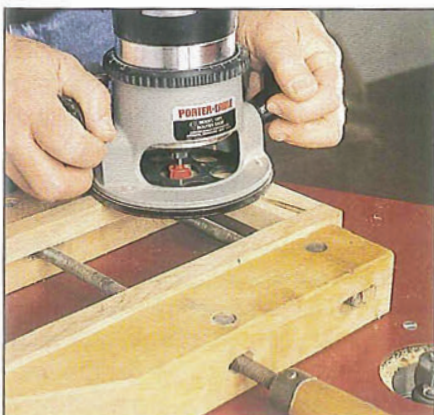
Photo F: Dry-clamp frames using large handscrew, then rout \frac{1}{8} " round-over on inside frame edges.
