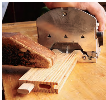
The side panels are the most complicated subassemblies of this project. To simplify it somewhat, the author used the Domino loose tenon joinery system from Festool.
