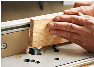
The author established the mortise locations in the breadboard ends, starting with a centered, stopped groove he cut on the router table.
