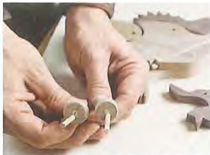
Figure 3: Offset the cam's axle by filling the boring created by the hole saw and drilling a second hole 3/16'' from the center.
