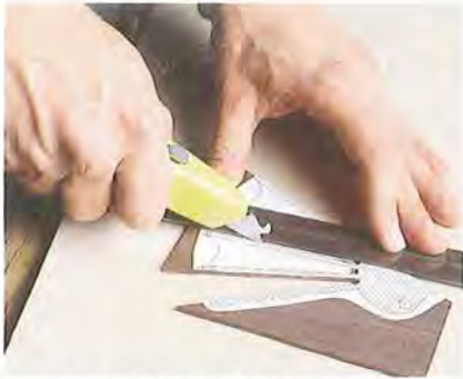
Figure 1: Lightly score the bones with a utility knife and a straightedge. Then hold the stock with the heel of your hand and complete the cuts with repeated firm knife strokes.
