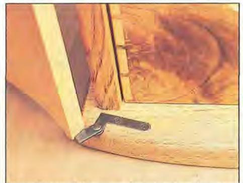
**Photo D:** Attach hinges to door, position door on cabinet, align both hinge leaves, and mark hinge location on the top and base. Then, cut cabinet gains as shown.
