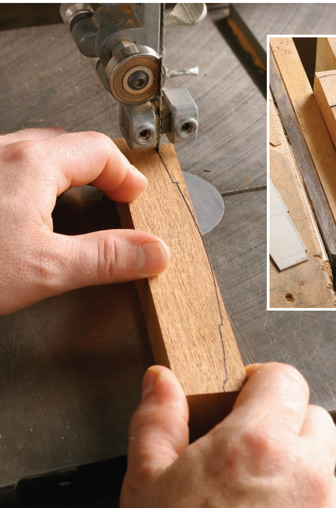
Forming the quartersawn mahogany drawer pulls is a time-consuming task. The author spent a significant number of hours detailing these pulls.
