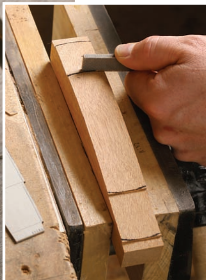
Forming the quartersawn mahogany drawer pulls is a time-consuming task. The author spent a significant number of hours detailing these pulls.
