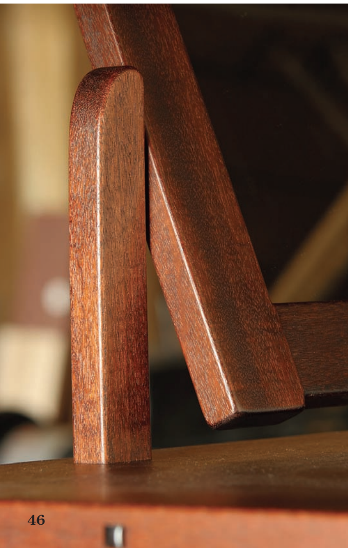
The posts of the mirror assembly are joined to the dresser top by screws driven up from the inside of the top. The top is attached to the carcass with tabletop fasteners.
