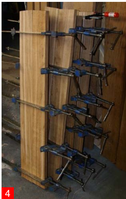
4. Begin selection with the longest boards. Here the sides are butt jointed and clamped together.
