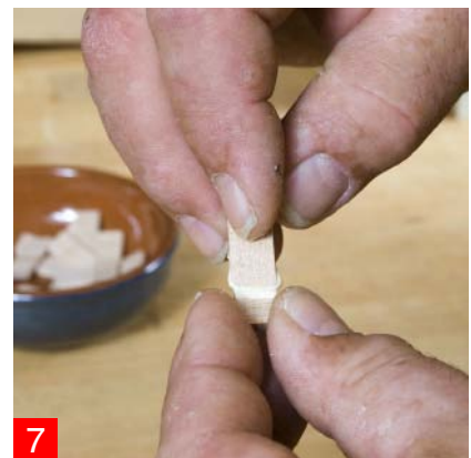
6 & 7. One person glues the wedges a pair at a time. Scrape glue on one wedge, then transfer by wetting the second from the first.
