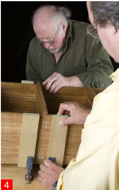
4 & 5. Setting up the clamps and clamping blocks requires working together as a team.
