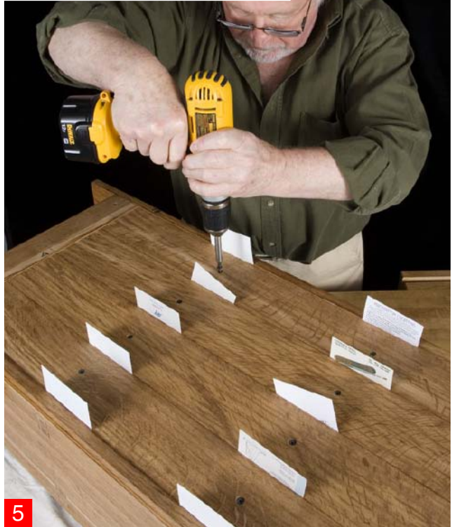
5. After the glue-up, equally space back slats with business cards and screw to shelves #2 and #3.
