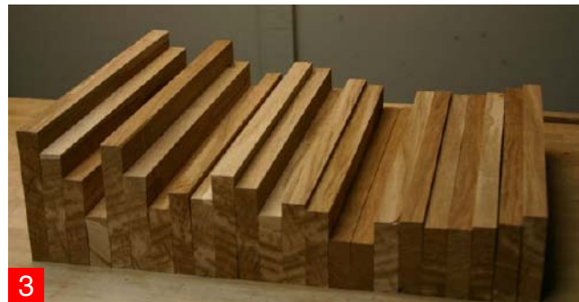
3. Shelf parts cut to length. The grain is straight and aligned with the edges. The remaining task is to make them into matching shelves 10" wide.
