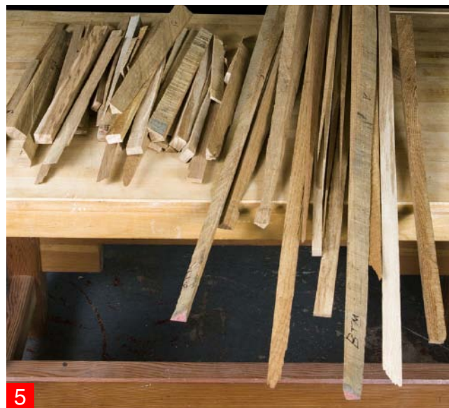
5. Here are some of the tapered cuts made in the quest for boards with the grain aligned with the edges.
