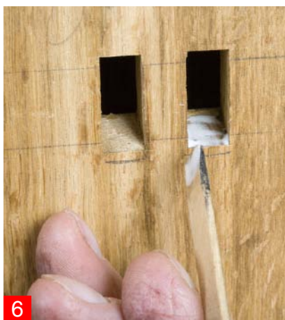
6 Apply glue to the end grain using a shaped spatula.
