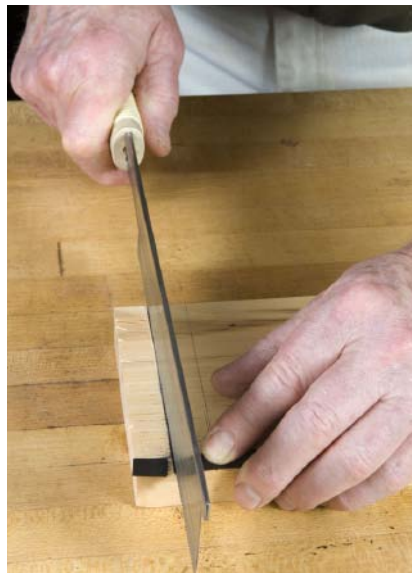
4 A kerf across the end of the shooting board simplifies cutting the veneer pieces to length.
