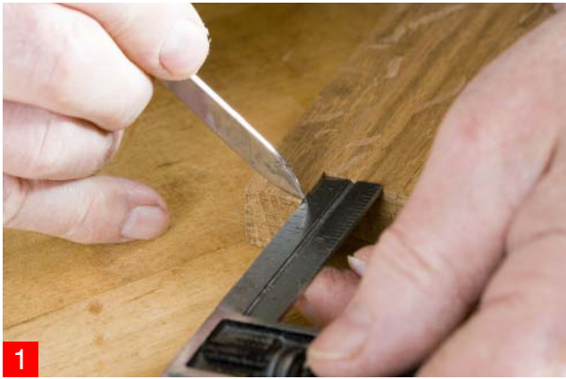
1 & 2. Knife around the shelf overhang at the correct length and angle.
