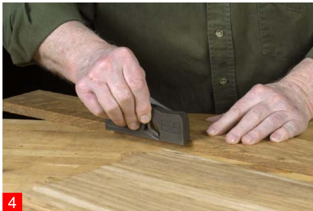
3 & 4. I used a small shoulder plane to clean up the rebates.
