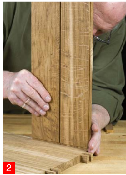
2. Check that the back slats fit easily into their grooves.
