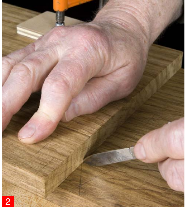
3 3. Set a mortise gauge to the knife marks and gauge the tenon. Then, with a marking gauge, gauge a line 1" from the front edge: the overhang will be marked accurately once the joint is entered. On the shelf overhang area, knife a line 5/8" from the shelf shoulder line to the 1" gauge line you just made. On the shelf, knife a line between the inside tenons 3/16" from the shoulder line. This will go into the housing between the mortises.
