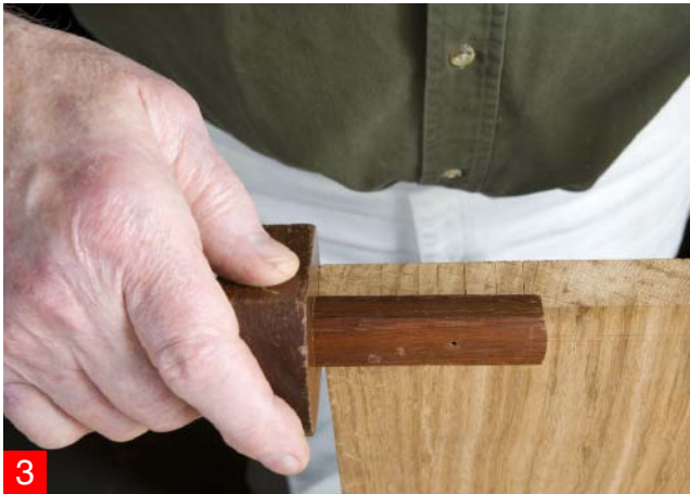
1 1. Mark the back edge mortise and tenons as normal and mark the front edge mortise.
