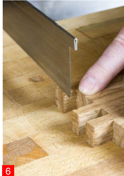
6. Saw to line with dozuki saw: fine kerf and slow cut.
