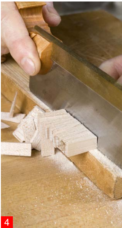
4. Lay the wedge stock on a sawing board and saw off all the wedges.
