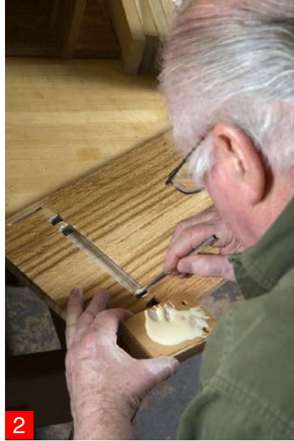
1 & 2. One person applies glue to the mortise parts while the other applies glue to the tenon pieces.
