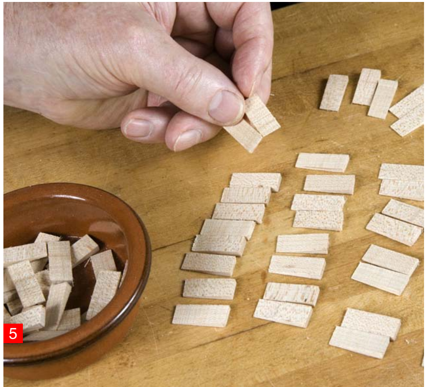
5. Collect and select the wedges. There will be size variations: just right, too big, and the odd one too small. Discard the too small. The too big are quickly corrected by putting the wedge against the end stop of a sawing board and removing the excess with a chisel.
