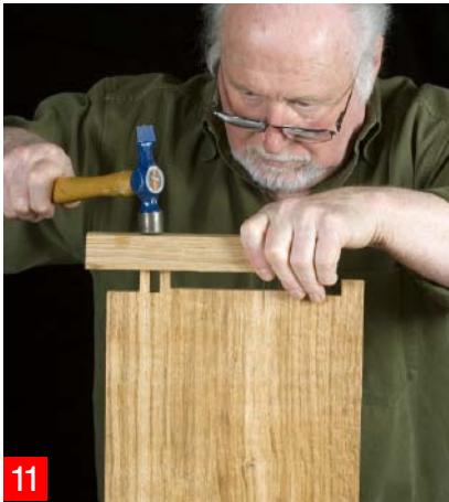
9 If you make a tiny chamfer on the edges of the shelf, it will enter the housing without getting hung-up.
