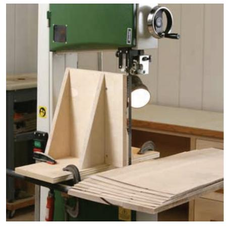
Using a rip fence on a band saw, like a rip fence you might find on a table saw, will nearly always cause grief - especially when you try cutting long boards. The fence alignment (which is pretty constant) fights the blade
