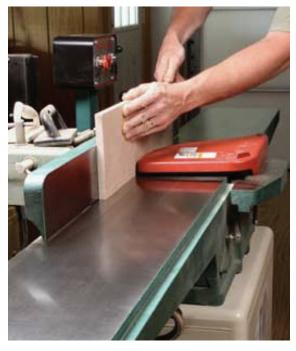
stock flat when you make the jointing pass, but it's simply returning to a sprung shape as soon as it leaves the cutters? Try taking gentler passes to start with, so the cutters knock off the ends but not the middle. Once the ends are in line with the center, you should be able to continue flattening without perpetuating a sprung edge. One other thing: it's tough to flatten the edges of long stock (say, 6 ft. or more). Practice on shorter lumber and see if your luck changes. It probably will.
