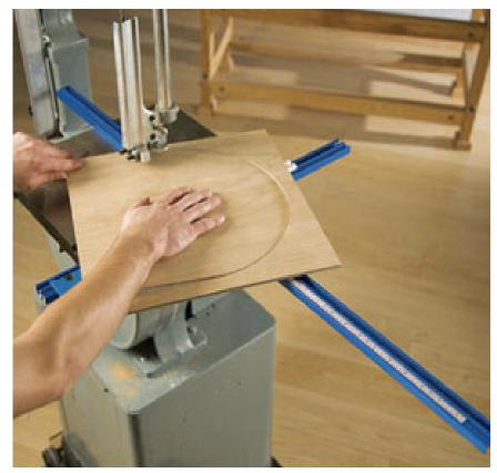
on the bottom to fit the miter gauge slot in my band saw fence. This lets me slide the jig and rough blank into the cut, much like a crosscut sled. When my jig hits the "stop" and is firmly in position, I can then finish cutting the circle.
