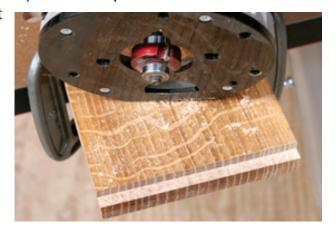
feel sharp -- or be 'brand-new,' the angles and edges are variable, and you might have a 'dull' bit. Test and compare. Sometimes the carbide on one side is way out of place relative to the carbide on another plane. With a little testing and observation - trial and error work - you can solve this problem. If I had to bet, it is the bit itself.
