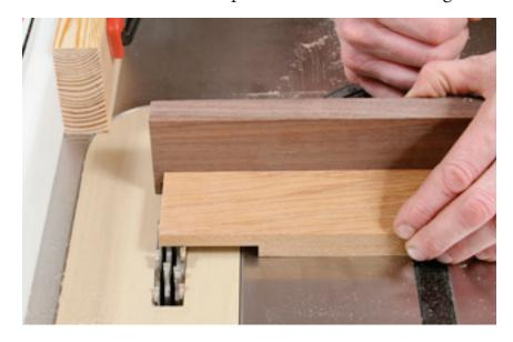
direction of the wood being cut (dado sets will cut dado joints across the grain, and plow joints with the grain) - all these factor into the operator's decision as to how deep the cut might be in order to have a clean, perfect, safe job. Setting a dado head to take out all the waste wood in one pass, and then ramming the boards across the saw at fast feed speeds, hell or high water, will not only result in a poor job, but extra wear and tear on the saw - and possibly the operator.
