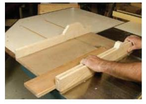
John Brock: Yes. I found I needed to run a fresh file down the sides of the miter slots in my table saw to remove a couple of rough spots. Then the UHMW polyethylene works well for miter guides. The only complaint is it will wear over time, depending on use and the roughness of your miter slots.
