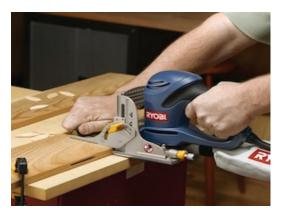
a nice, snug fit -- with multiple sources of biscuits. If I need a looser fit, I can manipulate the tool and make the groove sloppy. So from that, I can say the operator does have control over the fit. Maybe you're making multiple cuts on the same groove? Be sure the guide surfaces on the cutter are flat and seated before you plunge the cut.
