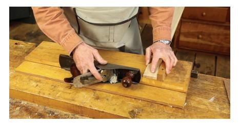
placed on the bench, the stuff to be planed placed on top and projecting out a 1/4" or so and clamped in place with clamps at the ends or with holdfasts or other clamping devices as appropriate.
