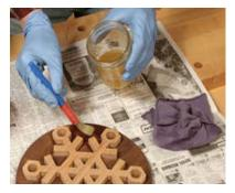
do is leave varnish-soaked or oily rags wadded up when they're still wet. As the finishes cure, they absorb oxygen and generate heat. If the finish gets hot enough in a crumpled rag, it can catch fire—and yes, it really happens. The simplest way to stay safe is to spread your rags out flat where they won't be disturbed until they fully cure and get hard. Then you can toss them in the trash.
