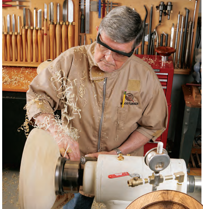
John Lannom turns the outside of a green bowl as it's held by the chuck. The wet shavings peel away in ribbons — a delightfully easy way to turn wood.
