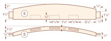
**Note:** the Lower Backrest Stretcher (piece 6) is the same as the Upper Backrest Stretcher (piece 5) except for the shaped top edge.
