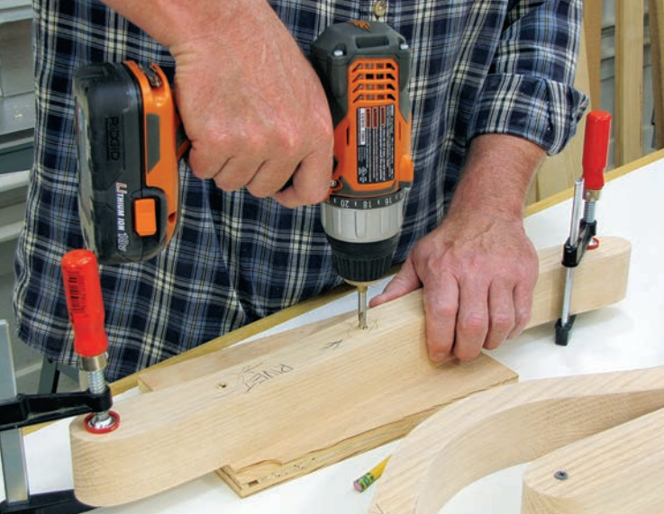
To make the task easier, clamp the component pairs together before removing the screws. To improve accuracy, use the screw holes as guides when you drill the rivet holes into the complex shaped pieces.
