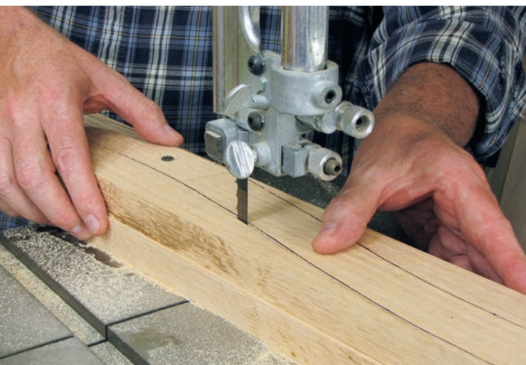
The best way to get identical parts for the pieces that come in pairs is to cut them simultaneously. Holes for the screws that hold the pieces together during machining are located where rivet holes will go later.
