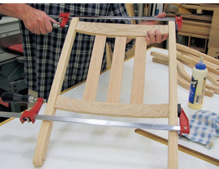
With glue applied to all joints, clamp up the backrest subassembly. When the glue has cured, you'll use the chair's completed backrest as a guide when you begin assembling the rest of the project.
