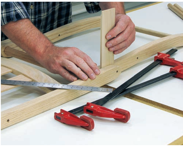
Sizing the leg set to exactly fit between the backrest members is critical. To allow for 1/8" on each side for washers, use a piece of 1/4" scrap as a feeler gauge. Adjust the length of rungs to give the leg set a perfect fit.
