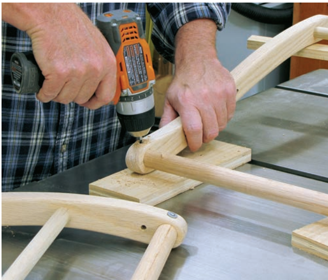
Drill a 3/16" hole through the ends of each seat stretcher, then install a rivet to create a rock-solid joint that simply won't come loose. This is the exact same joinery system that was used in the Civil War-era chairs.
