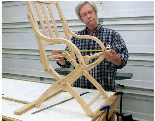
Use braces clamped to your work surface to keep the chair upright when taking seat measurements. Note the string tied around the stretchers — it'll keep the chair from collapsing should it slip out of the braces.
