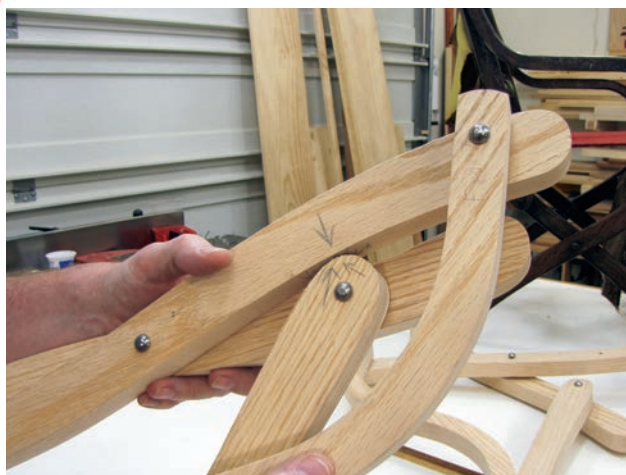
Temporarily insert rivets (photo above) to check the folding action to be sure nothing binds. The author cut the end of one leg just a hair too wide (photo right), causing the lower tip of the backrest to rub at the penciled-in arrows. A little more time on the spindle sander refined the leg to allow for clearance. (Note: rivets were purchased at www.rjleahy.com )
