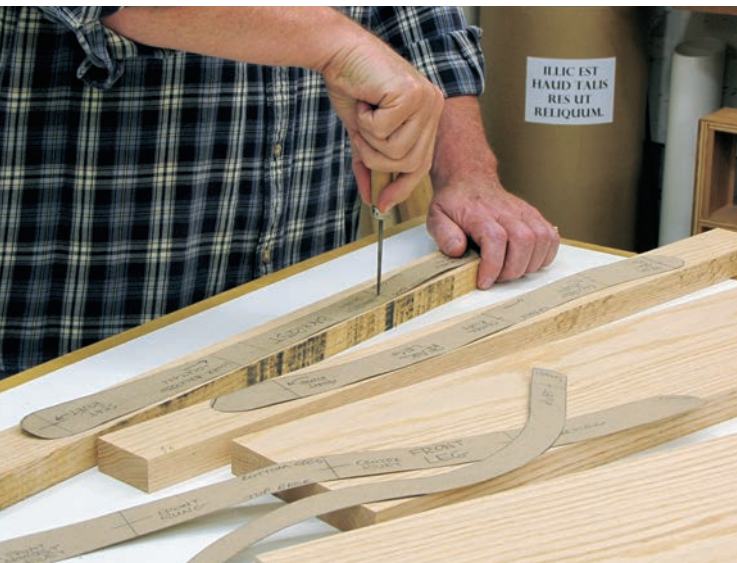
Lay out the component patterns to best match grain direction. The author used an awl punched directly through this pattern to accurately mark the locations for rivet holes. Time taken to make patterns is time well-spent.
