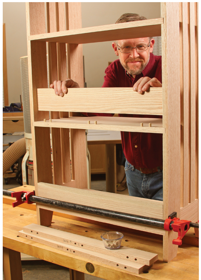
Step 22: With the bookcase dry-assembled, install the shelf backs on the shelves with the dowels in place to test the fit of these joints before gluing the parts together.
