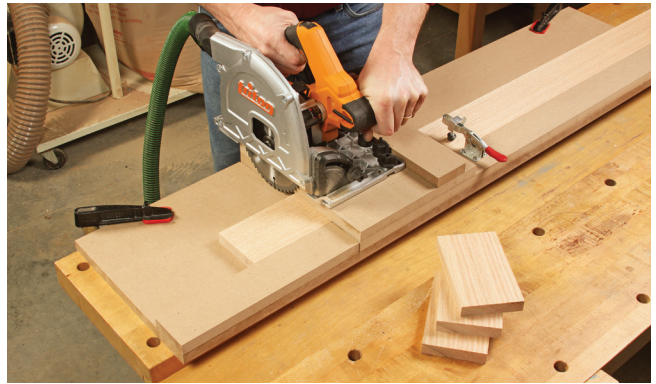
Step 3: Crosscut four side rails to length from a 1x4. This crosscutting jig (see page 4) makes the task easier to do accurately with a circular saw.
