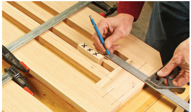
Step 9: Mark the side assemblies for single dowels that connect the stiles and rails. Center the dowel joints on the stiles.
