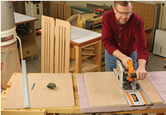
Step 14: Cut the four shelves to size from a 2 x 4-ft. oak plywood "handy panel." Guide your circular saw with a clamped straightedge, or use a track if your saw has one, to ensure that these cuts are straight.
