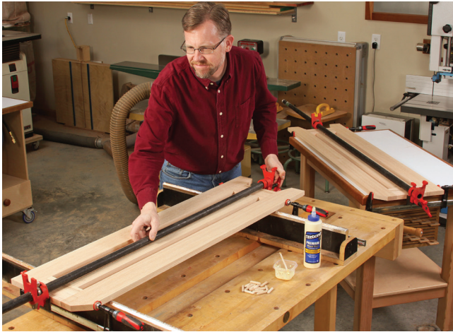
Step 12: Glue and clamp the side assemblies together. Start with the rail and stile joints, then add the legs, working your way from the innermost joints outward.
