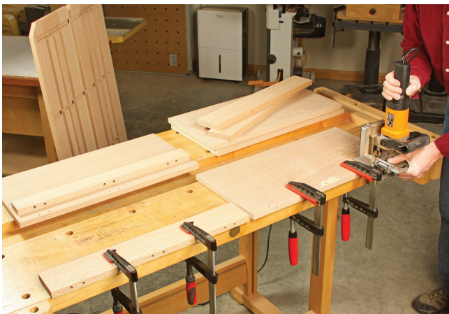
Step 21: Create dowel joints between the shelves and shelf backs, using at least three dowels. The Triton Duo Dowel Jointer shown here drills pairs of holes spaced 1¼" apart.
