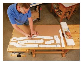
You can create full-size tracing patterns by enlarging the gridded drawings on the second page of this PDF. Rockler also offers a kit (shown above) containing all the cardboard patterns you'll need to build this bench project. Either way, full-size patterns are an essential part of the building process.
