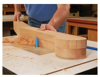
Rigid templates will help you reproduce this bench's curved and angled shapes at the router table. Here, the template is mounted to the bottom of this bench leg workpiece as it's being template-routed to final shape. Make your templates from 1/4" hardboard, plywood or MDF, using your full-size patterns to trace the template shapes.
