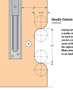
Laying out the handle cutouts is really just a matter of joining pairs of 1½"-dia. circles on each end of the shape: a quarter of one circle's circumference forms the outer curve of the cutout, and one quarter of the adjacent circle forms the inner curve. Make these handle cutouts at least 4" wide or as needed to suit your hand size.
