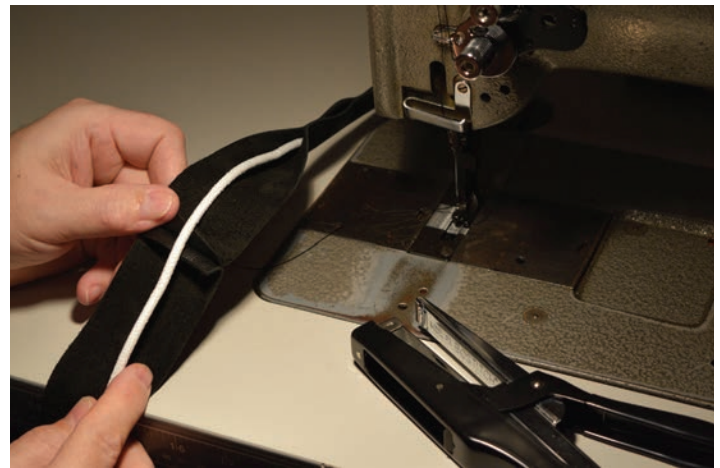
The author joined leather strips together to achieve the required length of piping. Open the seams and lay them flat before sewing.
