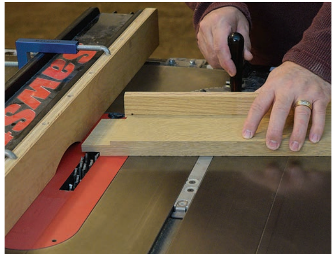
Angle a miter gauge and cut the tenon cheeks with a dado blade. You’ll know the angle is correct when the rail ends sit flush against the rip fence. Sneak up on the blade height until the tenon fits into the mortise.
