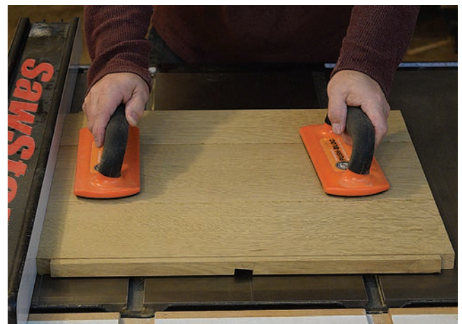
Form an angled dado in the side panels with a single pass. Stack the dado to 7/8 " wide, and tilt it to 6.5^\circ for this cut.
