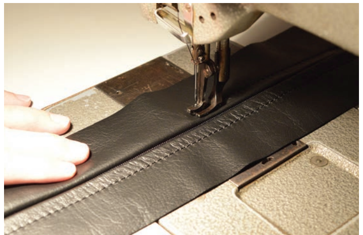
Finally, topstitch on each side of the zipper. Slightly close the leather gap to conceal the zipper for a clean appearance.
