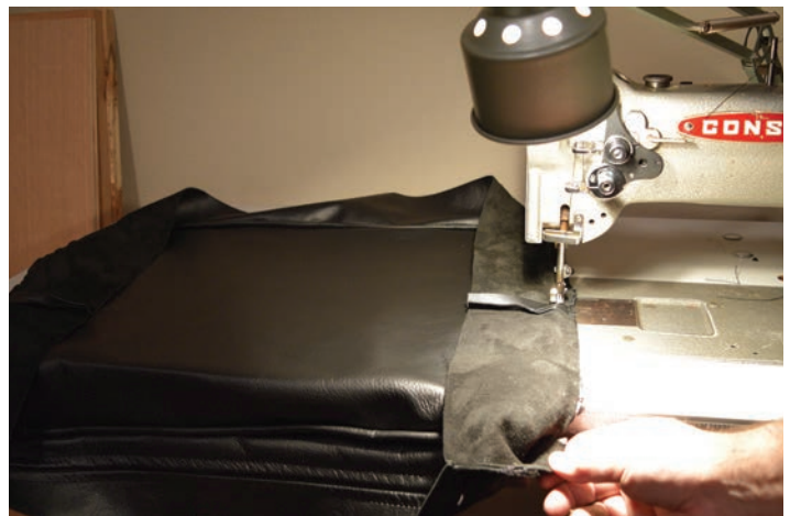
With a 1/4" cording foot installed on the sewing machine, stitch the top plate to the boxing strip. The cording foot follows the piping like a train on tracks. Then repeat this stapling and sewing process for the bottom plate.
