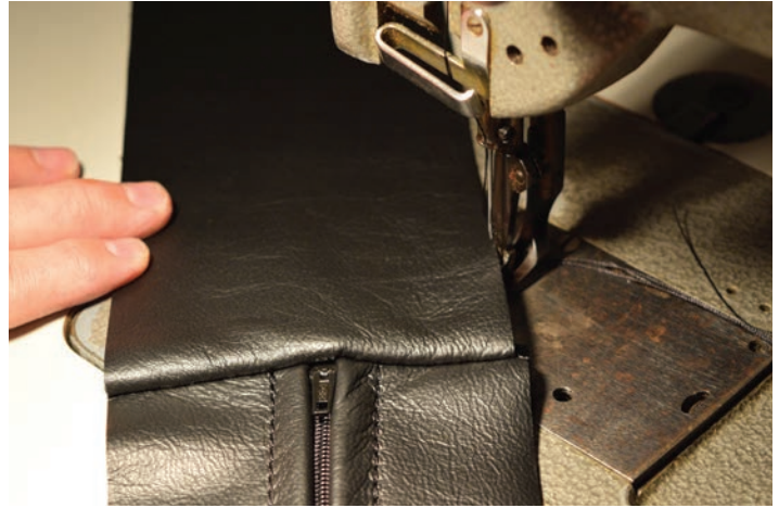
Build the cushion piece by piece. Attach the boxing strip to the zipper panel with a blind stitch.
