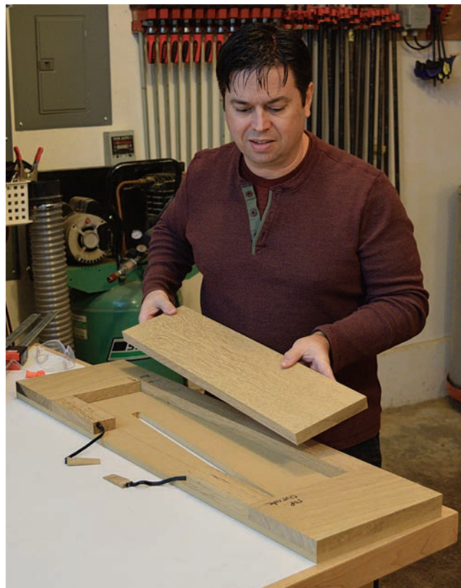
The author secures leg blanks in the routing jig with wedges. He's tacked the wedges to the jig with leather straps so they're always close at hand.
