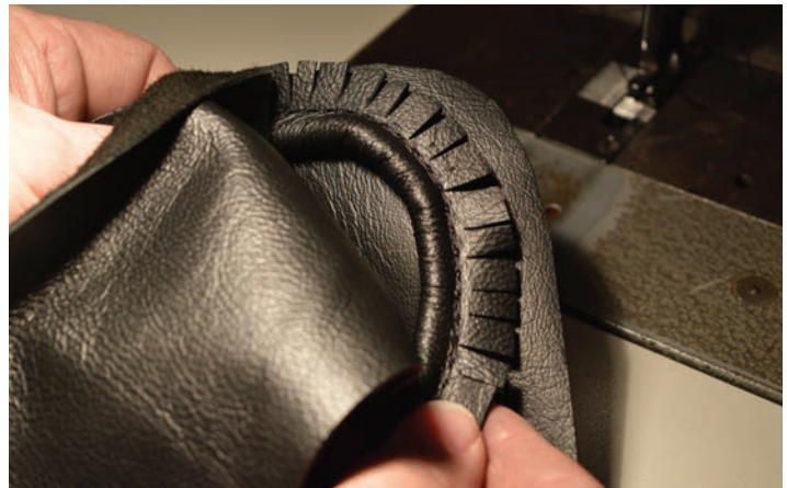
Cut nicks in the piping for smoother corners. Then staple the piping between the top plate and boxing strip.
