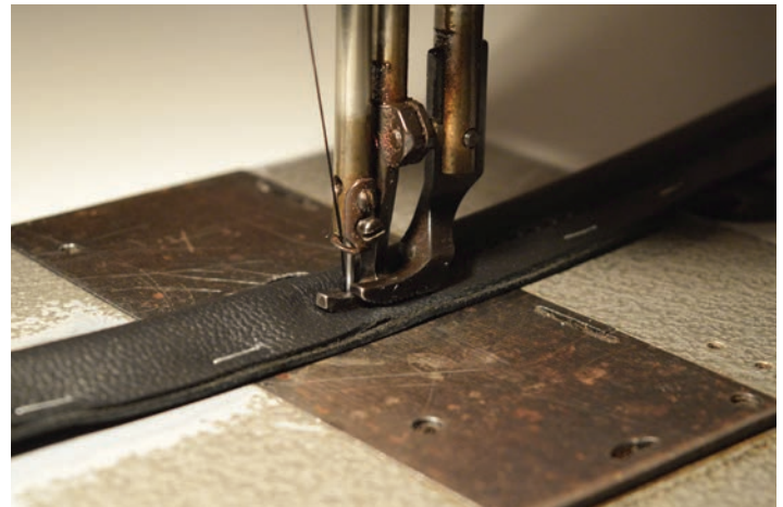
If you're a beginner behind a sewing machine, use a stapler to wrap the leather strips around the cording. With a zipper foot on the sewing machine, sew right next to the cord.
