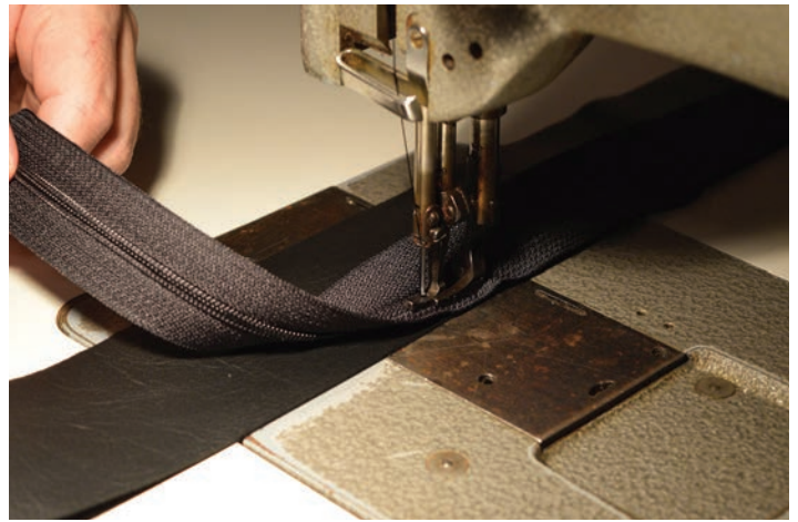
Zipper panel in three easy steps. Cut a length of zipper a little longer than needed, and blind sew it to one of the zipper panel strips. For this first step, you'll be sewing right along the zipper teeth.
