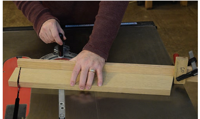
With a miter gauge locked at 10.5°, miter one end of the front and back rails. Then use a stop block clamped to an auxiliary fence to cut a matching angle on the other end.
