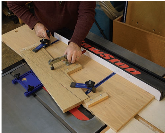
Secure the leg blanks to a tapering sled to rip their inside edges to 10.5^\circ . A low profile featherboard can help hold the sled against the fence.
