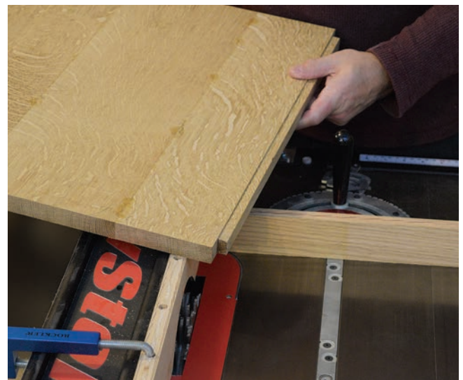
Raise stub tenons on the side panels. Trim their end cheeks and shoulders until the tenons fit the leg grooves snugly.
