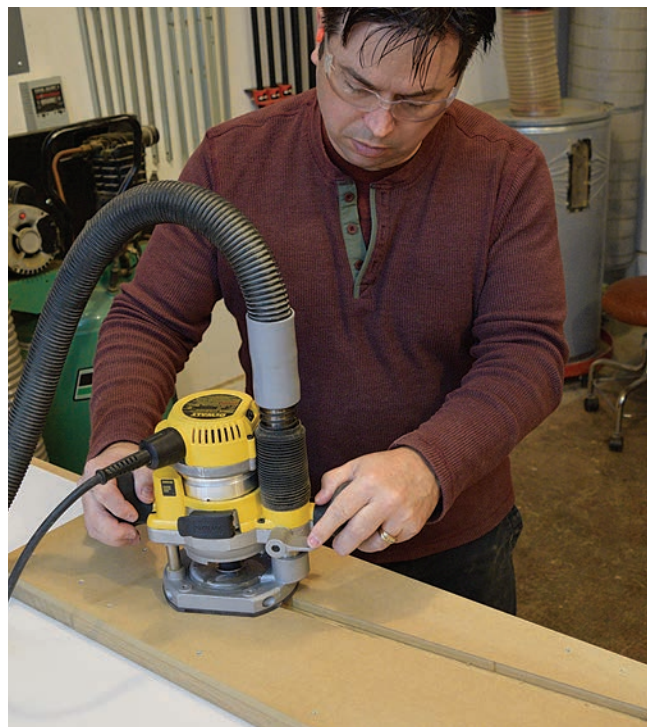
Clamp the jig in place and rout an angled groove in each leg. The jig fully supports the router for a predictable, accurate cut.
