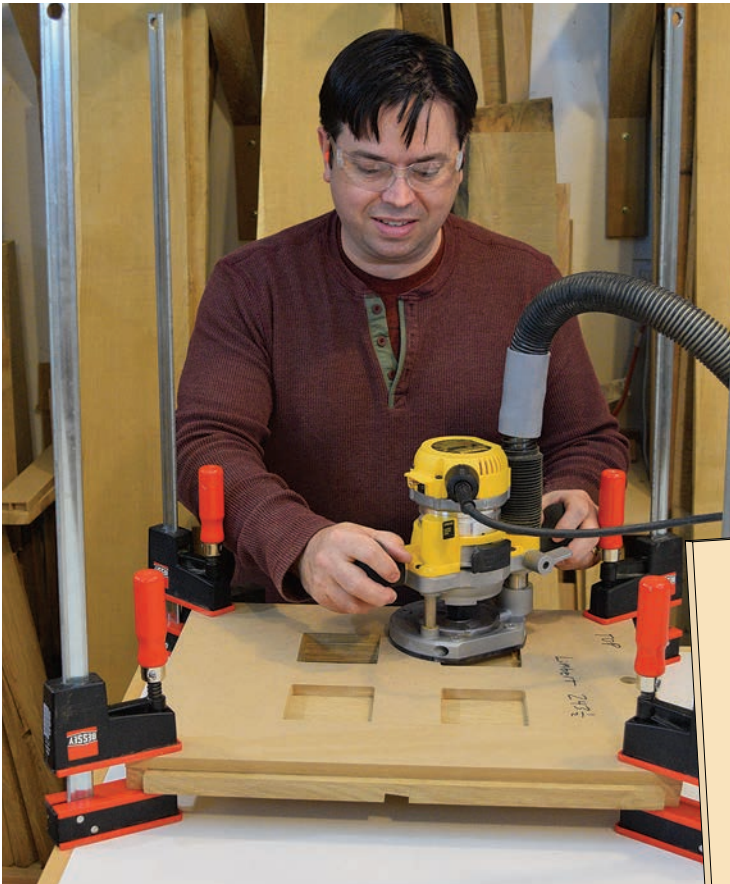
Clamp the template on top of the side panel, and rough out the squares with a router equipped with a guide bushing and spiral bit.
