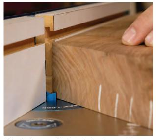
With a 5/8"-diameter straight bit chucked into the router table, we cut a 1/4" x 1/4" rabbet along the straight edge of each tabletop piece. This step commits which faces of the parts will be the show faces.
