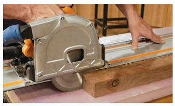
While the outer edges of the tabletop are irregular, its inner edges must be straight. Ripping these inner edges straight was easy to do with a track saw, but a regular circular saw and a straightedge guide will also work well.
