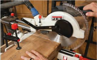
Once the tabletop sections were marked on the long stock, it was broken down into more manageable blanks at the miter saw with square crosscuts. Mitering the parts would come later, after surfacing.
