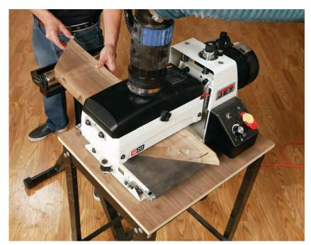
JET's compact 10/20 Drum Sander proved to be more than up to the job of surfacing the tabletop parts. It has all the features of its bigger siblings with a smaller footprint. Here, the tabletop pieces are sanded to remove any stray machining marks and surface tearout.
