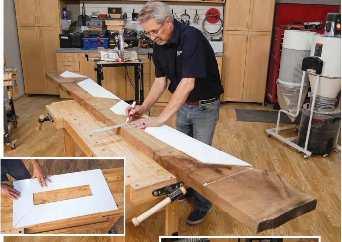
Mitered templates for each tabletop section helped locate the workpieces relative to the board's waney edges while also giving us a preliminary idea of how the parts would come together (inset).
