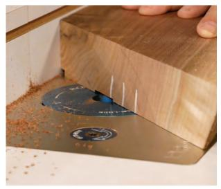
Here, a 1/16"-deep by 1"-wide groove is plowed into each tabletop component to accept the inlay strips. Using a 5/8"-diameter straight bit, two passes are required to achieve the 1" width.
