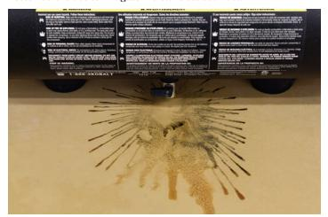
All compressors accumulate condensed water, which can rust a compressor's tank if not drained regularly. Drain it by opening a valve on the bottom of the tank. It's good practice to drain the tank after every use.
