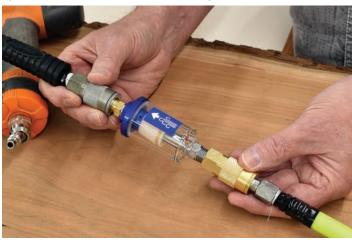
To keep liquids from entering tools, an inline filter – installed between the compressor and tool – helps minimize the amount of water traveling through the hose.
