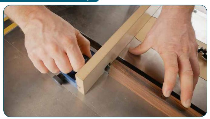
The rest of the cross lap notches are cut using the Cross Lap Jig. Set the width of the jig's indexing keys to match the thickness of the slats.
