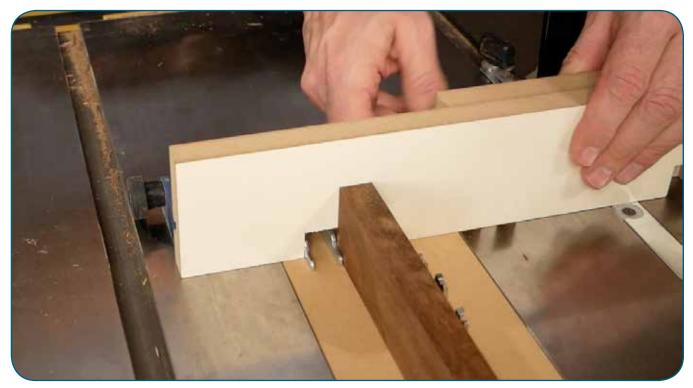
Reposition the jig fence to cut the notches in the Short Slats. Leave the dado set at the same height. Use one of the slats as a gauge to adjust the distance between the indexing keys and dado set to match the width of the slats.
