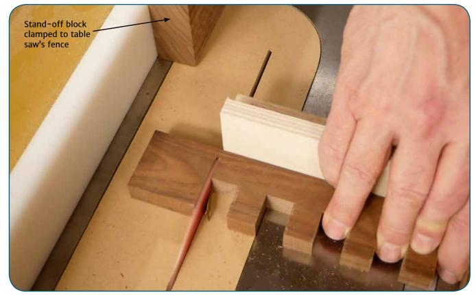
Trim the excess length off of all slats. Clamp a stand-off block to the fence a few inches in front of the blade. Next, position the fence and stand-off block so that the blade is lined up to cut flush with the edge of the last notch.
