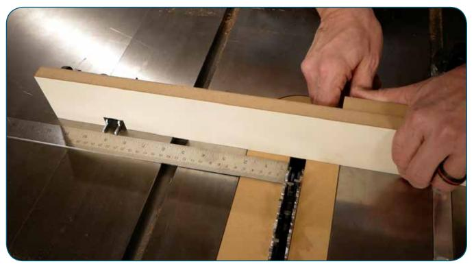
To set up to cut the second and subsequent notches on the 14 Long Slats, adjust the jig fence so that the inside edge of the indexing keys is  $8^1/2^{11}$  from the edge of the dado set.
