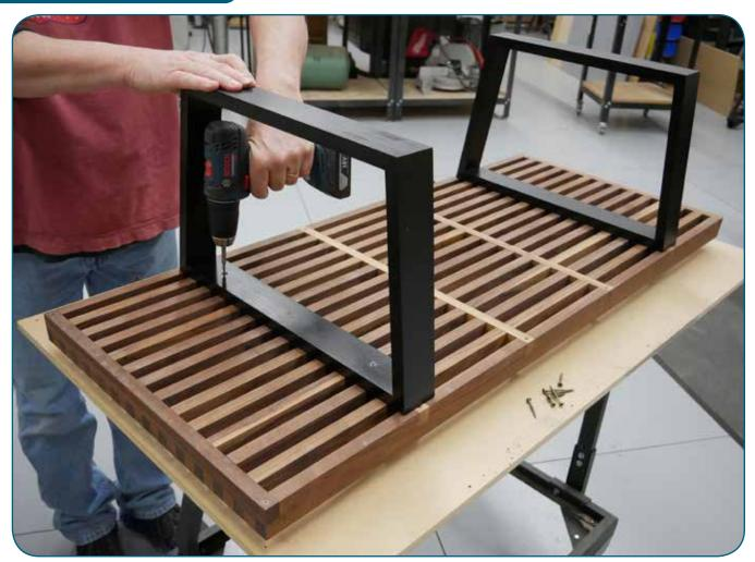
Position the leg assemblies as shown and drill countersinks and pilot holes for  $\#8 \times 1^{1}/_{2}$ " screws. Attach the leg assemblies to the table top with the screws.
