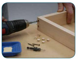
Cut the leg parts to size. Drill counterbores and pilot holes for  $\#8 \times 1^1/2^{11}$  screws at connection points. Assemble the legs with glue and screws. Conceal the screw holes with wood plugs.
