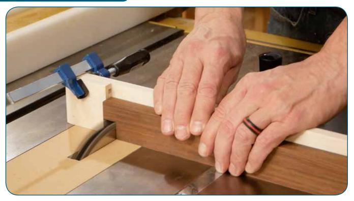
All slats require a notch cut flush with the very end at one end. Clamp a stop block to a miter gauge to position the slats to cut the end notches on all slats.
