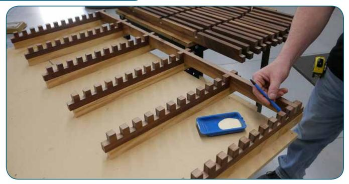
Lay out the Short Slats on the bench with their notches up. Apply glue to the bottom of the notches. Then place each inside Long Slat over the Short Slats, carefully aligning the notches. Do not attach the outer Long Slats at this point.
