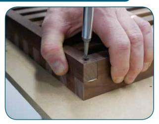
The outer Long Slats are the most vulnerable to detaching, so these slats are glued on and the joints are reinforced with screws. Apply glue to the notches and fit the outer Long Slats onto the Short Slats. To avoid splitting the wood, drill pilot holes and countersinks for #6 x 1-1/4" screws into each cross lap joint on the outer Long Slats and secure the slats with the screws.
