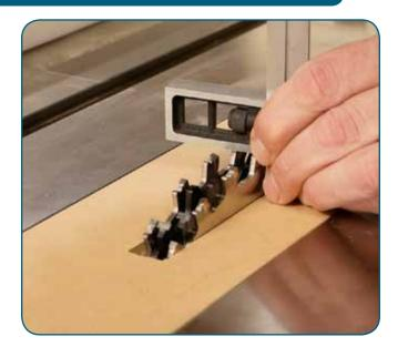
Install a dado set in your table saw. Set the width of the dado set to match the thickness of your workpieces. Set the height at 7/8". Make test cuts on scrap pieces to test the fit of the cross lap joint. Adjust the dado height and width if the joint is not fitting properly.
