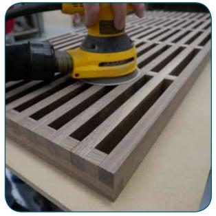
After the glue has cured, remove the clamps and sand the surfaces flush. Apply Danish oil to any surfaces that are unfinished.
