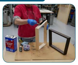
Dye the legs black with dye stain. We used an alcohol-based stain. Apply a topcoat after the stain is dry.
