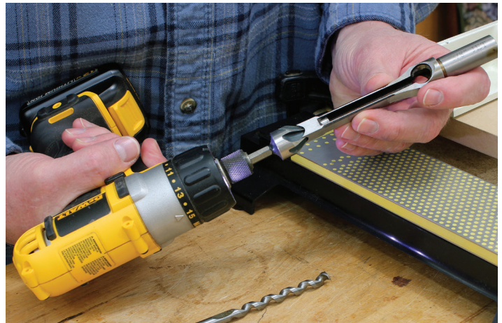
Photo 1. In order to be effective, mortising chisels must be kept as sharp as possible. Honing is a two-step process. First, use a simple sharpening bit in a handheld drill/driver to hone the inside of the bit. Then, complete the honing by rubbing all cutting edges over a flat sharpening surface — like the diamond sharpener shown here — to remove burrs.
