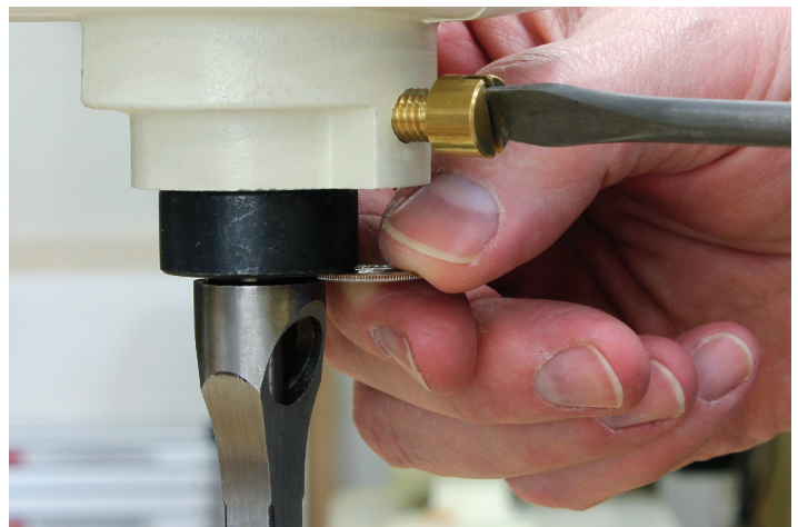
Photo 2. To ensure that a mortising chisel's auger spins slightly ahead of the chisel cutting edges, use a dime as a spacer when installing or changing bits. Once the auger distance is set, remove the dime and snug the hollow chisel firmly up against the quill.
