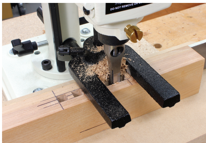
Photo 4. After first defining the mortise ends, a series of overlapping square holes completes the mortise. The horseshoe-shaped hold-down keeps the workpiece firmly on the table when retracting the chisel.
