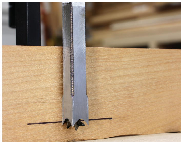
Photo 3. To allow plenty of room for a tenon to seat properly, the chisel depth is set slightly below the tenon length before setting the depth stop. Here, the author has marked a line indicating tenon length, then set the cutting end of the chisel approximately 1/8" below the line.
